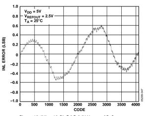
Figure 13. INL—12-Bit DAC, 2.5 V Internal Reference
