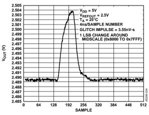
Figure 34. Digital-to-Analog Glitch Impulse (Negative)
