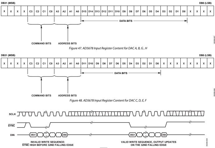
Figure 49. SYNC Interrupt Facility
