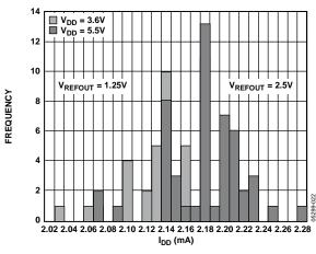
Figure 22. IDD Histogram with Internal Reference
