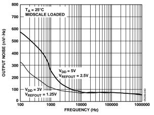
Figure 40. Noise Spectral Density, Internal Reference
