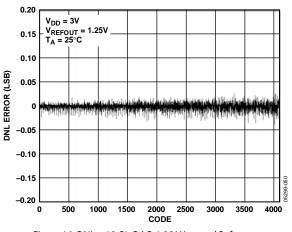
Figure 16. DNL—12-Bit DAC, 1.25 V Internal Reference
