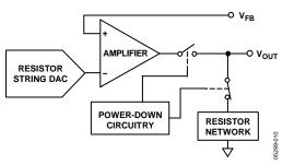
Figure 50. Output Stage During Power-Down
