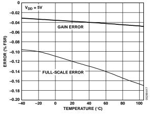
Figure 17. Gain Error and Full-Scale Error vs. Temperature
