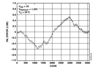
Figure 15. INL—12-Bit DAC, 1.25 V Internal Reference
