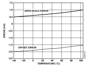
Figure 18. Zero-Scale Error and Offset Error vs. Temperature
