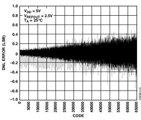
Figure 8. DNL 16-Bit DAC, 2.5 V Internal Reference
