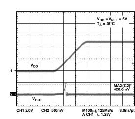
Figure 31. Power-On Reset to 0 V
