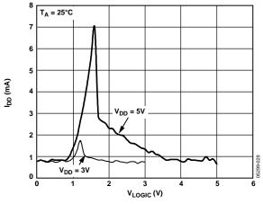
Figure 29. Supply Current vs. Logic Input Voltage
