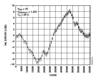
Figure 9. INL—16-Bit DAC, 1.25 V Internal Reference
