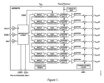
The outputs of all DACs can be updated simultaneously using the  $\overline{\text{LDAC}}$  function, with the added functionality of user-selectable DAC channels to simultaneously update. There is also an asynchronous  $\overline{\text{CLR}}$  that clears all DACs to a software-selectable code—0 V, midscale, or full scale.
