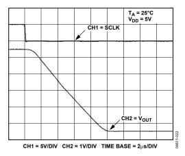
Figure 22. Full-Scale Settling Time
