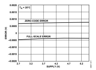
Figure 11. Zero-Code/Full-Scale Error vs. Supply at 25°C
