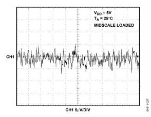
Figure 27. 1/f Noise, 0.1 Hz to 10 Hz Bandwidth
