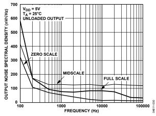
Figure 30. Noise Spectral Density
