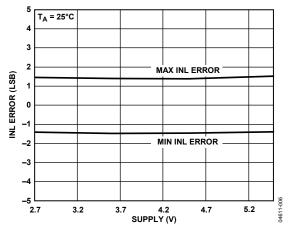
Figure 6. INL Error vs. Supply at 25°C
