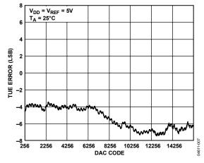
Figure 7. Typical Total Unadjusted Error (TUE)
