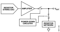
Figure 36. Output Stage During Power-Down
