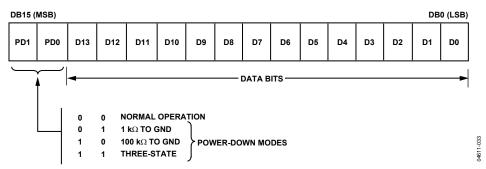
Figure 34. Input Register Contents
