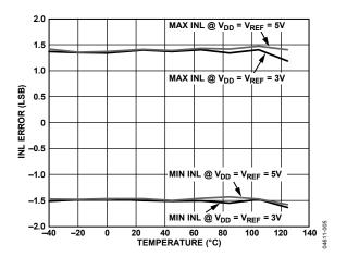
Figure 5. INL Error vs. Temperature (3 V/5 V Supply)
