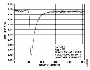
Figure 26. Digital-to-Analog Glitch Energy
