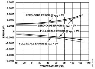
Figure 10. Zero-Code/Full-Scale Error vs. Temperature (3 V/5 V)
