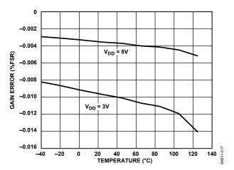
Figure 17. Gain Error vs. Temperature (3 V/5 V)
