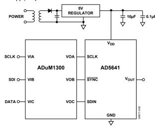
Figure 44. AD5641 with a Galvanically Isolated Interface
