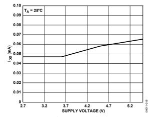
Figure 19. Supply Current vs. Supply Voltage at 25°C
