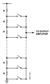
Figure 33. Resistor String Structure
