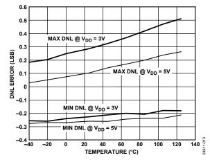
Figure 13. DNL Error vs. Temperature (3 V/5 V)
