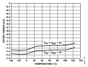
Figure 16. Offset Error vs. Temperature (3 V/5 V Supply)
