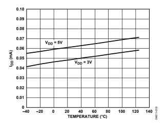
Figure 18. Supply Current vs. Temperature (3 V/5 V Supply)
