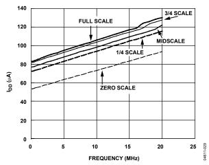
Figure 29. IDD vs. SCLK vs. Code
