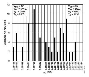
Figure 15. I<sub>DD</sub> Histogram (3 V/5 V)
