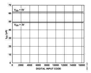
Figure 21. Supply Current vs. Digital Input Code
