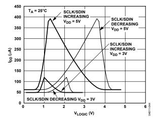
Figure 31. SCLK/SDIN vs. Logic Voltage
