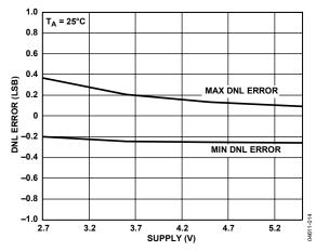
Figure 14. DNL Error vs. Supply at 25°C
