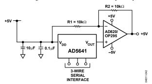
Figure 43. Bipolar Operation with the AD5641
