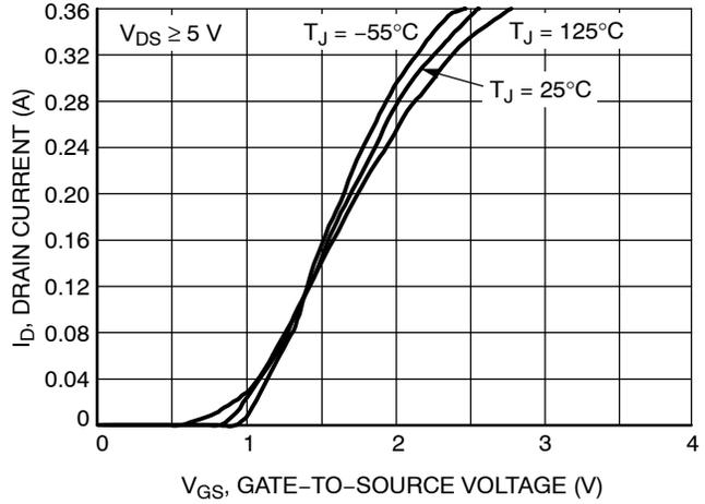
Figure 2. Transfer Characteristics
