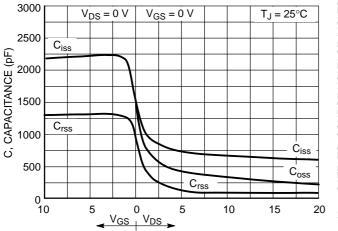
GATE-TO-SOURCE OR DRAIN-TO-SOURCE VOLTAGE (VOLTS)
