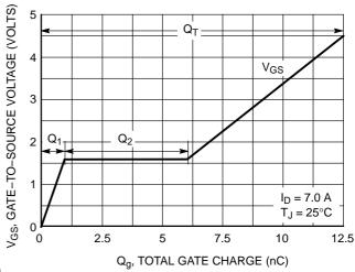
Figure 8. Gate-to-Source Voltage versus Total Charge
