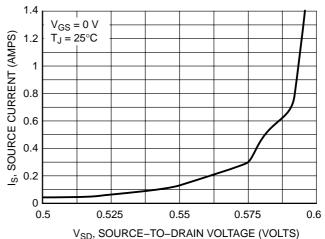
Figure 10. Diode Forward Voltage versus Current
