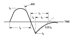
Figure 12. Diode Reverse Recovery Waveform
