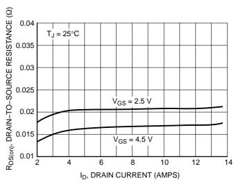
Figure 3. On–Resistance versus Gate–to–Source Voltage
