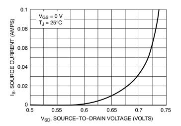
Figure 9. Diode Forward Voltage vs. Current
