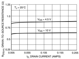
Figure 3. On-Resistance vs. Drain Current and Temperature
