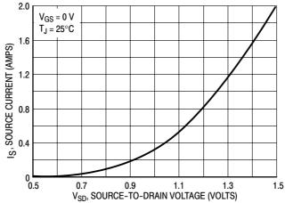
Figure 10. Diode Forward Voltage versus Current
