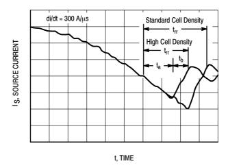
Figure 11. Reverse Recovery Time (t<sub>rr</sub>)
