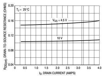
Figure 3. On–Resistance versus Gate–To–Source Voltage
