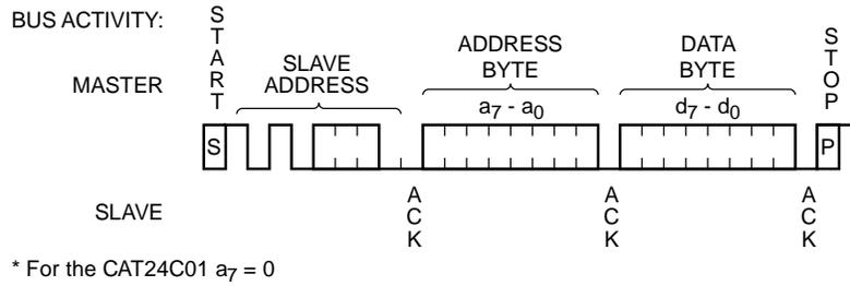
Figure 6. Write Cycle Timing
