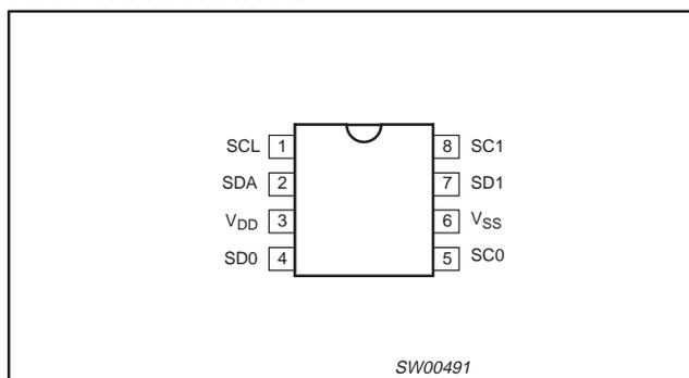
Figure 1. Pin configuration
