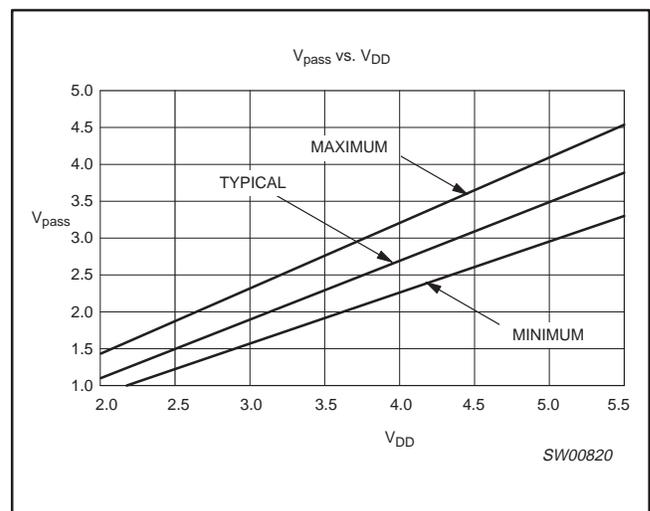
Figure 5. V<sub>pass</sub> voltage
