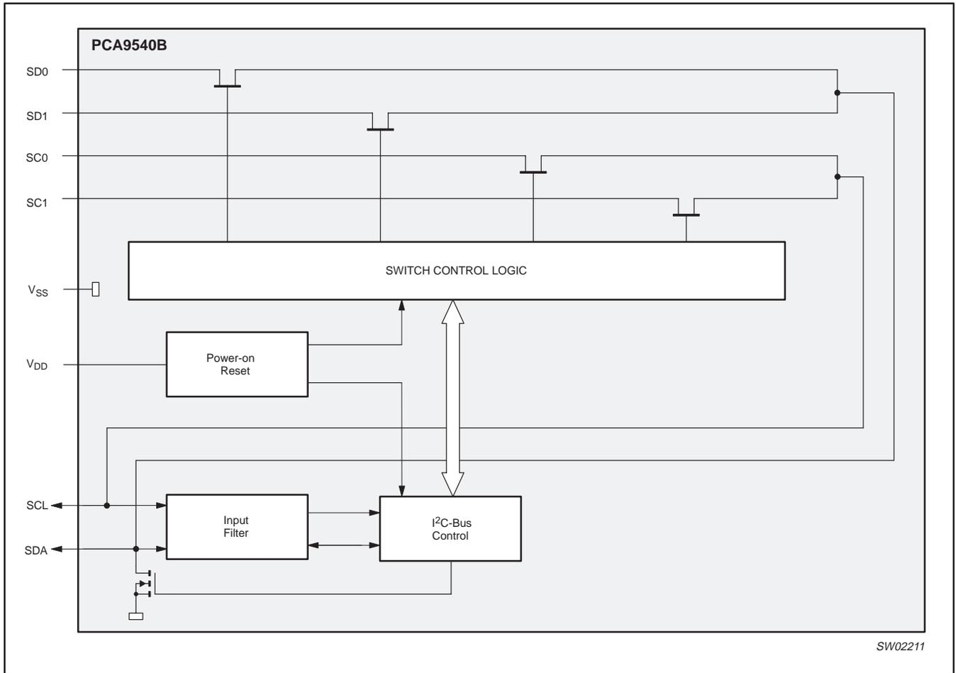
Figure 2. Block diagram
