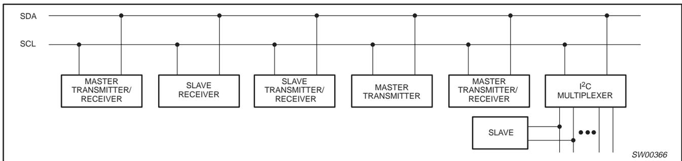
Figure 8. System configuration
