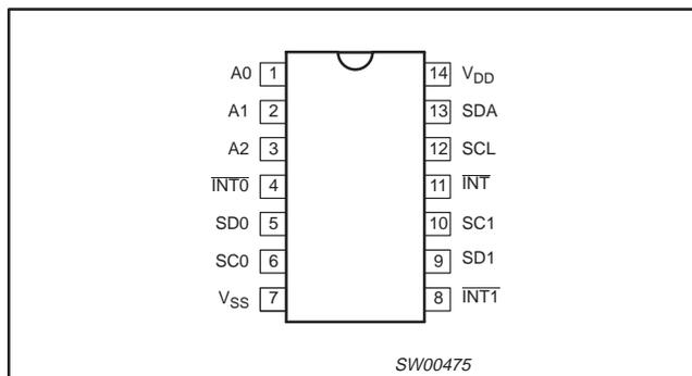
Figure 1. Pin configuration
