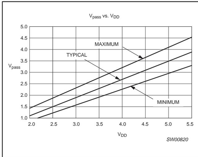
Figure 5. V<sub>pass</sub> voltage
