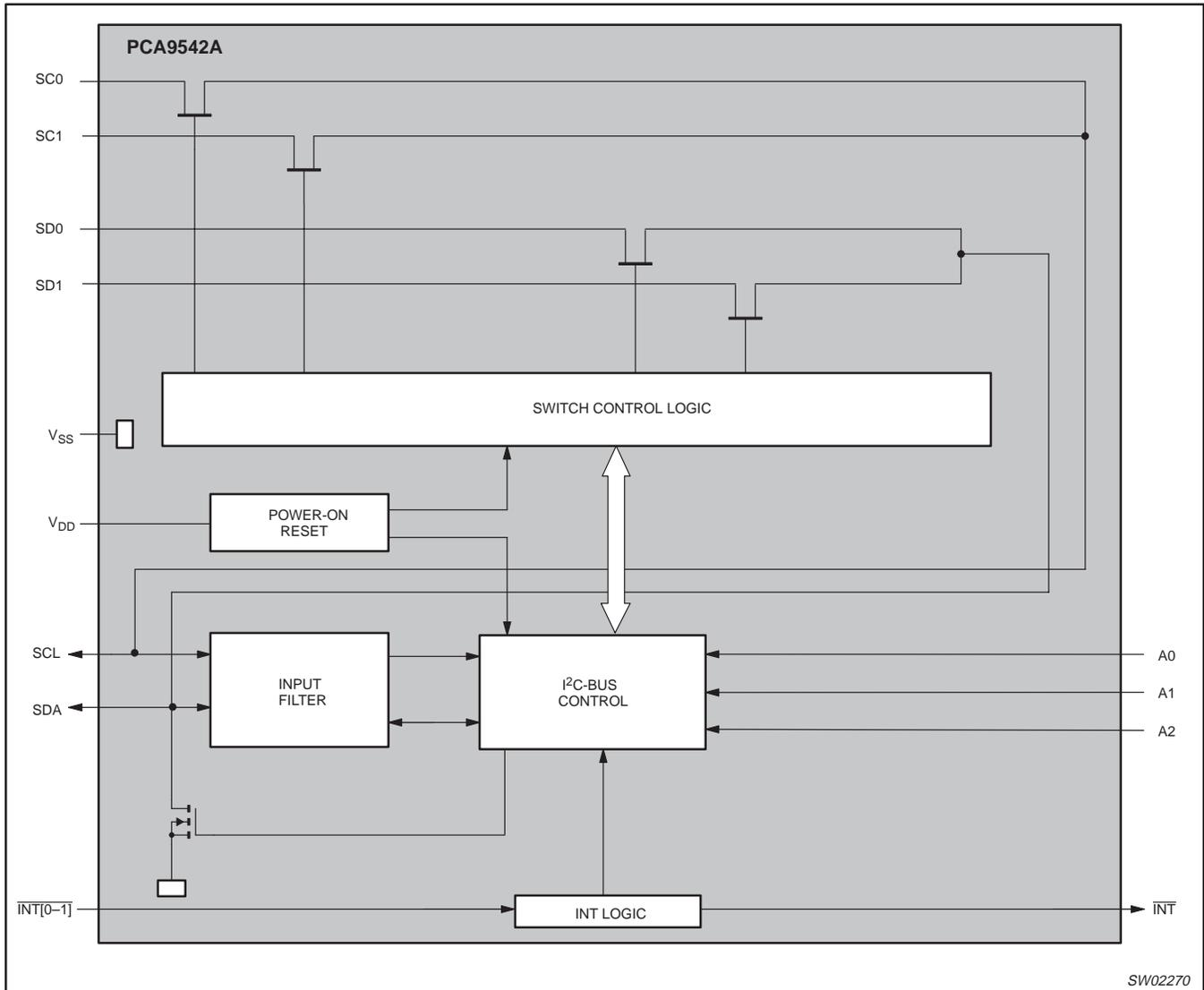
Figure 2. Block diagram
