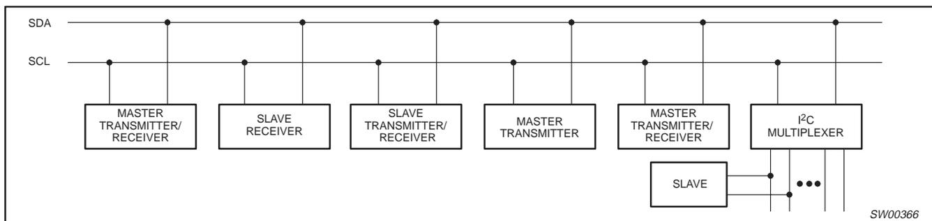
Figure 8. System configuration
