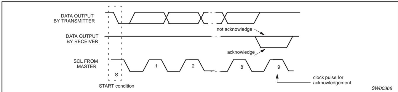
Figure 9. Acknowledgement on the I<sup>2</sup>C-bus
