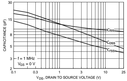
Figure 8. Capacitance Characteristics.
