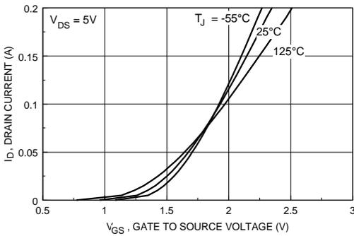
Figure 5. Transfer Characteristics.
