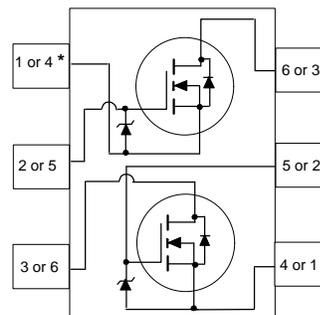
\* The pinouts are symmetrical; pin 1 and 4 are interchangeable.
