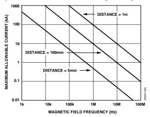
Figure 20. Maximum Allowable Current for Various Current-to-ADuM240x Spacings
