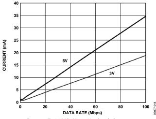
Figure 14. Typical ADuM2401  $V_{\rm DD2}$  Supply Current vs. Data Rate for 5 V and 3 V Operation
