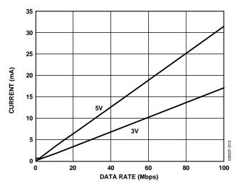
Figure 13. Typical ADuM2401  $V_{\rm DD1}$  Supply Current vs. Data Rate for 5 V and 3 V Operation
