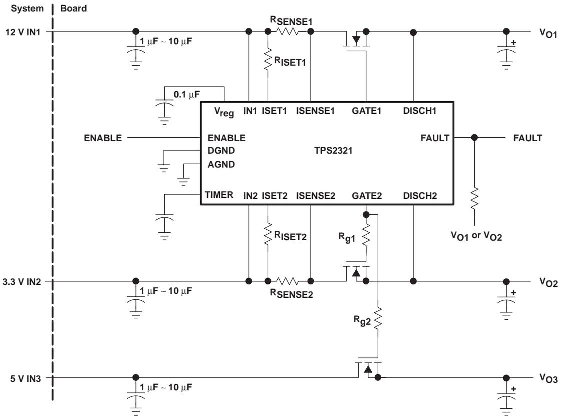
Figure 27. Three-Channel Application
