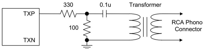
Figure 16. Consumer Output Driver Circuit
