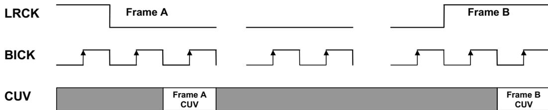
Figure 7. Audio routing, DIF modes 5 and 7 (I<sup>2</sup>S)
