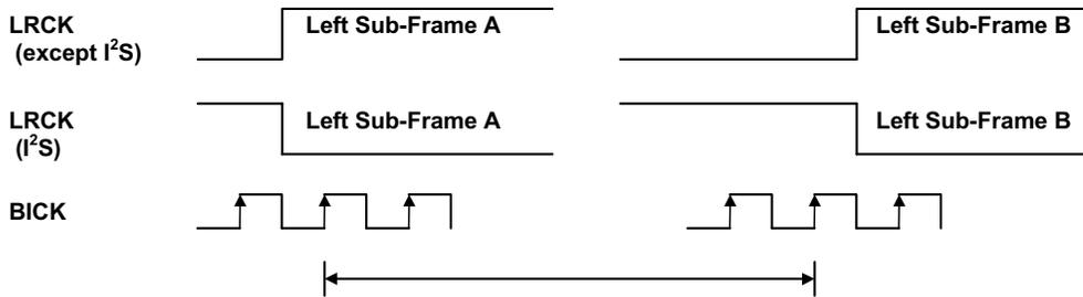
Figure 3. Block start timing in audio routing mode
