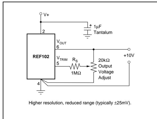
FIGURE 4. REF102 Optional Output Voltage, Fine Adjust.
