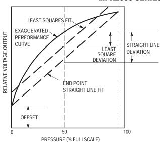
Figure 2. Linearity Specification Comparison
