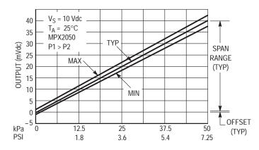
Figure 3. Output versus Pressure Differential
