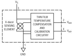
Figure 1. Temperature Compensated Pressure Sensor Schematic
