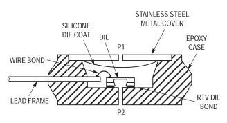
Figure 4. Cross-Sectional Diagram (not to scale)
