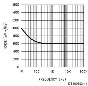
**Typical Performance Characteristics** To generate these curves the LM62 was mounted to a printed circuit board as shown in Figure 2. (Continued)
