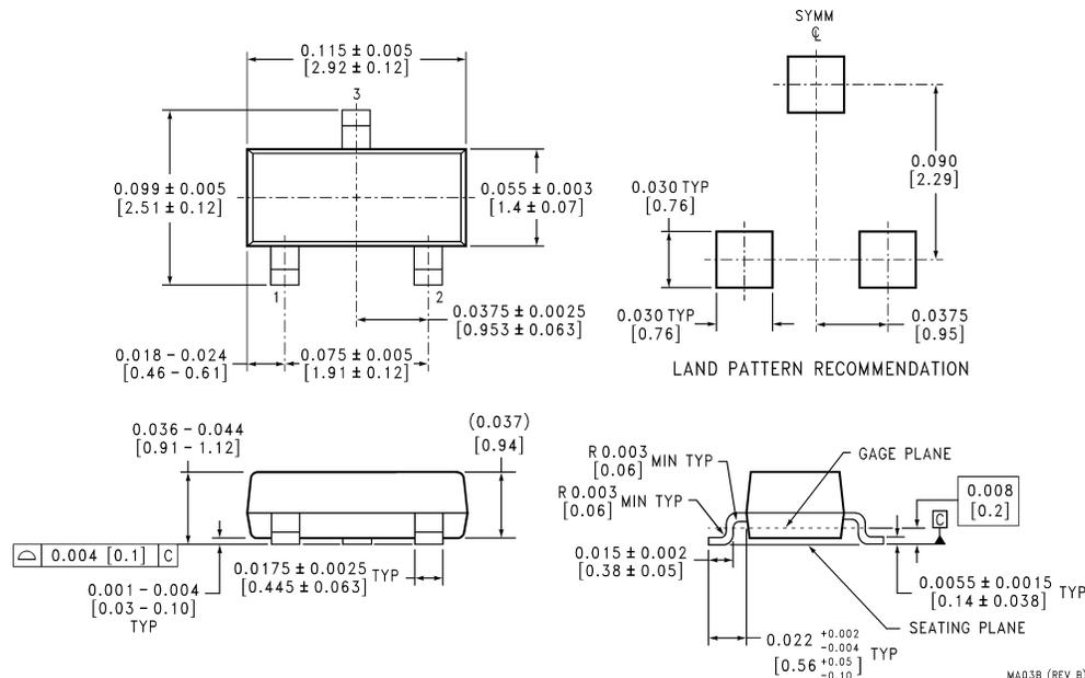
**SOT-23 Molded Small Outline Transistor Package (M3)**
