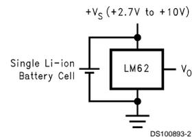
$$V_O = (+15.6 \text{ mV/}^\circ\text{C} \times T^\circ\text{C}) + 480 \text{ mV}$$
