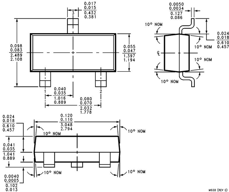
**SOT-23 Molded Small Outline Transistor Package (M3)**
