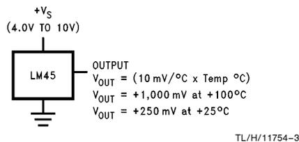
**FIGURE 1. Basic Centigrade Temperature Sensor ( $+2.5^\circ\text{C}$  to  $+100^\circ\text{C}$ )**
