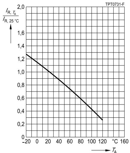
**Characteristics (typical) for  $T_{ref} = 120\text{ }^{\circ}\text{C}$**
