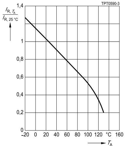
**Characteristics (typical) for  $T_{ref} = 130\text{ °C}$**
