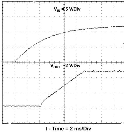
Figure 19. Startup Waveform,  $V_{in}$  and  $V_{out}$ .
