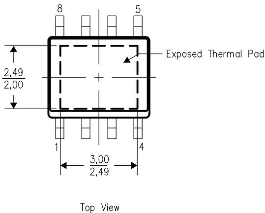
NOTE: All linear dimensions are in millimeters
