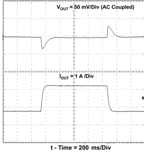
Figure 18. Transient Response,  $I_o$  Step 0.75 to 2.25 A.
