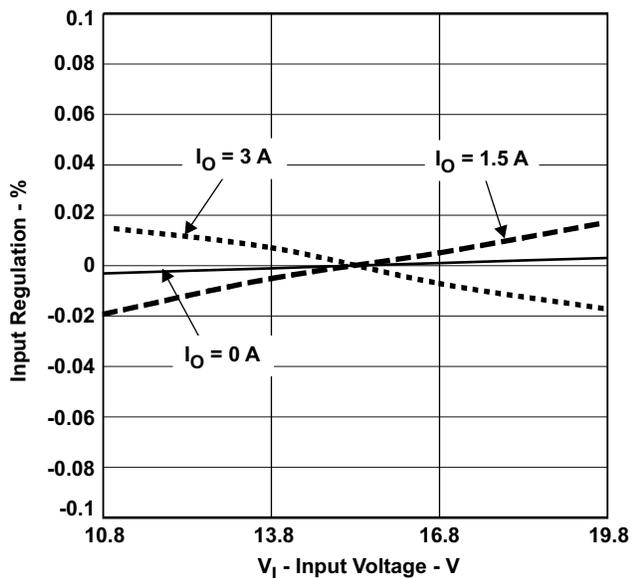
Figure 15. Input Regulation % vs. Input Voltage
