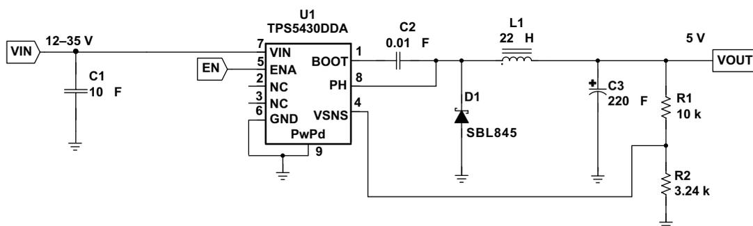
Figure 12. 12-35 V Input to 5 V Output Application Circuit
