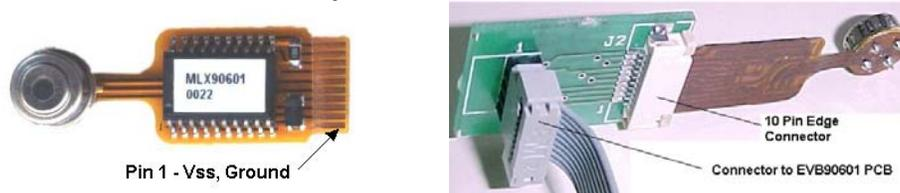
3. Connect the ribbon cable to the large pcb and the small pcb
