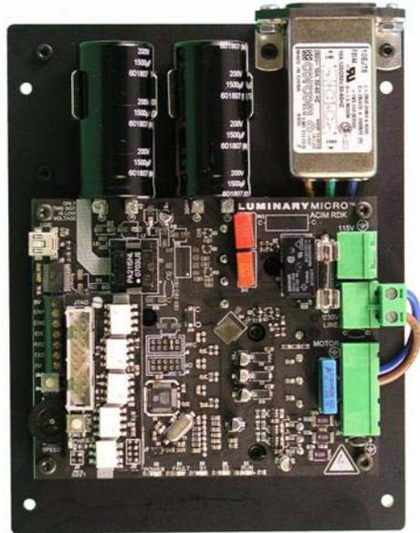
Figure 2. ACIM RDK Control Board
