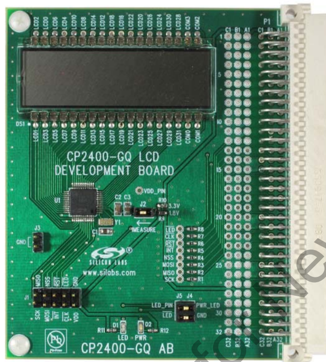
Figure 3. CP2400 Development Board
