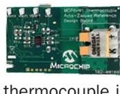
The MCP6V01 design board demonstrates how to use a difference amplifier system to measure Electromotive Force (EMF) voltage at the cold junction of thermocouple in order to accurately measure temperature of the thermocouple bead. This can be done by using the MCP6V01 auto-zeroed op amp because of its ultra low offset Voltage (VOS) and high Common Mode Rejection Ratio (CMRR).
