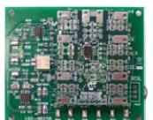
The MCP651 Input Offset Evaluation board is intended to provide a simple means to measure the MCP651 Input Offset Evaluation Board op amp's input offset voltage under a variety of operating conditions. The measured input offset voltage (VOST) includes the input offset voltage specified in the data sheet (VOS) plus changes due to: power supply voltage (PSRR), common mode voltage (CMRR), output voltage (AOL), input offset voltage drift over temperature ( $\Delta$ VOS/ $\Delta$ T) and 1/f noise.
