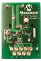
The MCP1640 Synchronous Boost Converter Evaluation board demonstrates the MCP1640 in two boost-converter applications with multiple output voltages. It can be used to evaluate both package options (SOT-23-6 and 2x3-8 DFN). This board was developed to help engineers reduce the product design cycle time.
