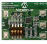
The MCP73871 Demo Board with Voltage Proportional Current Control is designed to demonstrate Microchip's stand-alone linear Li-Ion battery charger with system power path and load sharing management control solution. The MCP73871 integrates the required elements to meet design challenges when developing new Li-Ion/Li-Polymer batteries powered products.
