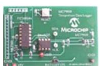
Allows users to store up to 128,000 temperature readings from the MCP9800 sensor to the 24LC1025, Microchip's 1024 Kbit EEPROM. A PIC16F684 MCU communicates with the sensor and EEPROM. In addition, the PIC MCU interfaces to a PC using the PICkit™ 1 Flash Starter Kit and transfers the temperature readings from the EEPROM to the PC. Microsoft Excel® can be used to view the data.
