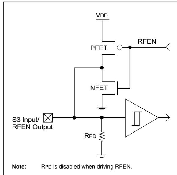
**FIGURE 2-5: DATA PIN DIAGRAM**
