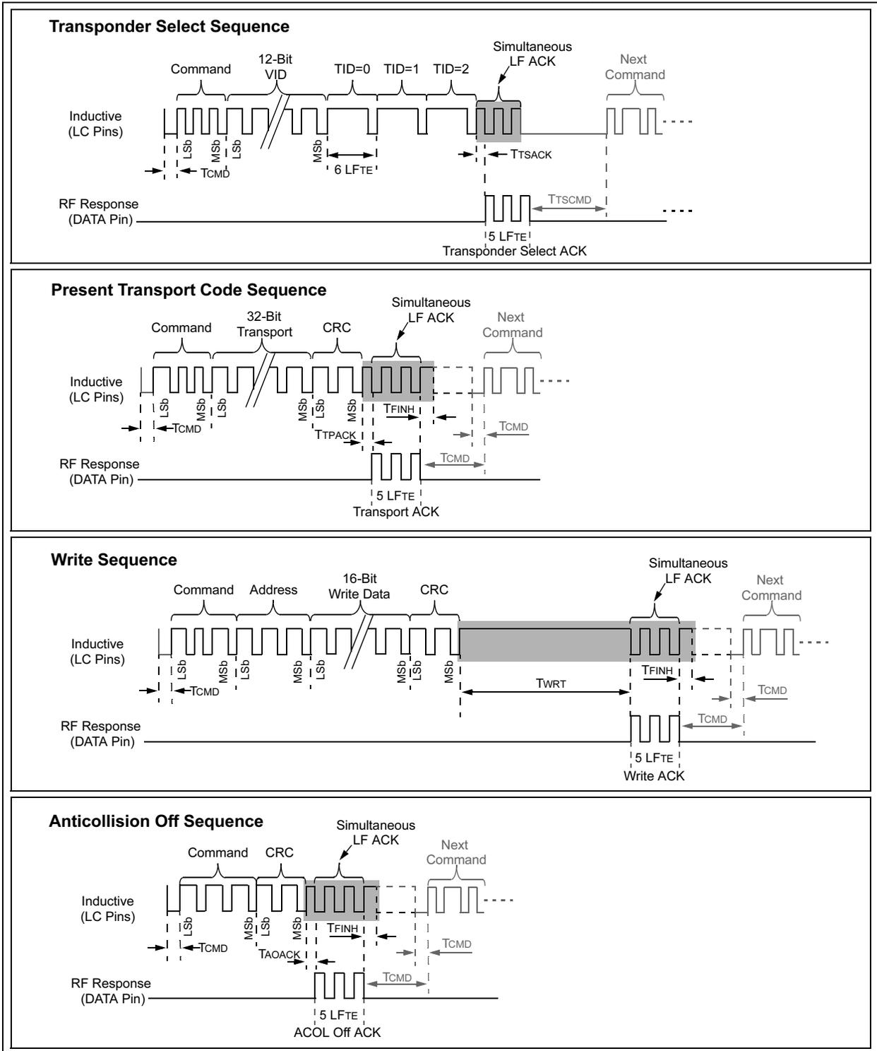
**FIGURE 3-20: LF DATA RESPONSE ADJUSTMENTS (LFRSP=1)**
