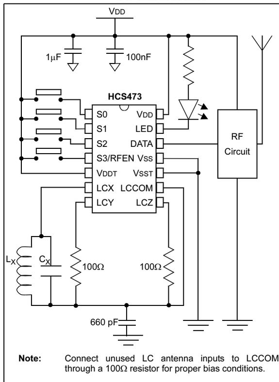
**FIGURE 2-3: S0/S1/S2 PIN DIAGRAM**
