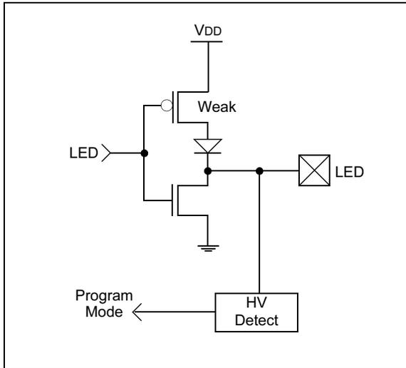
**FIGURE 2-7: LCCOM/LCX/LCY/LCZ/VSST PIN DIAGRAM**
