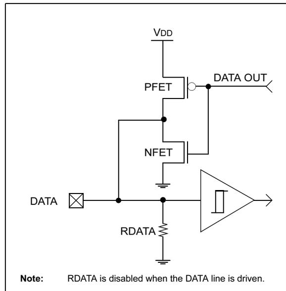
**FIGURE 2-6: LED PIN DIAGRAM**
