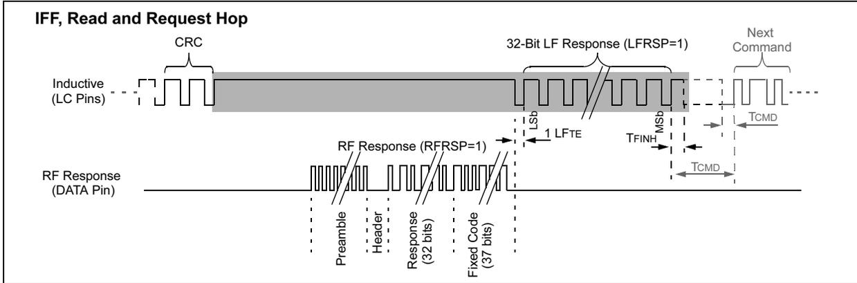
**FIGURE 3-21: LF COMMUNICATION ANALOG DELAYS**
