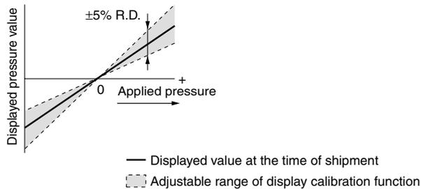
Note) When the display calibration function is used, the regulating pressure value may change  $\pm 1$  digit.
