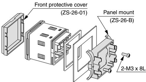
Tighten screws 1/4 to 1/2 turn after the heads are flush with the panel.
