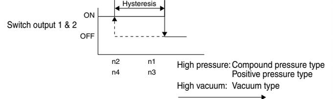
Note) If the hysteresis is set for less than 2 digits, the switch output may possibly chatter when the input pressure changes around the set value.
