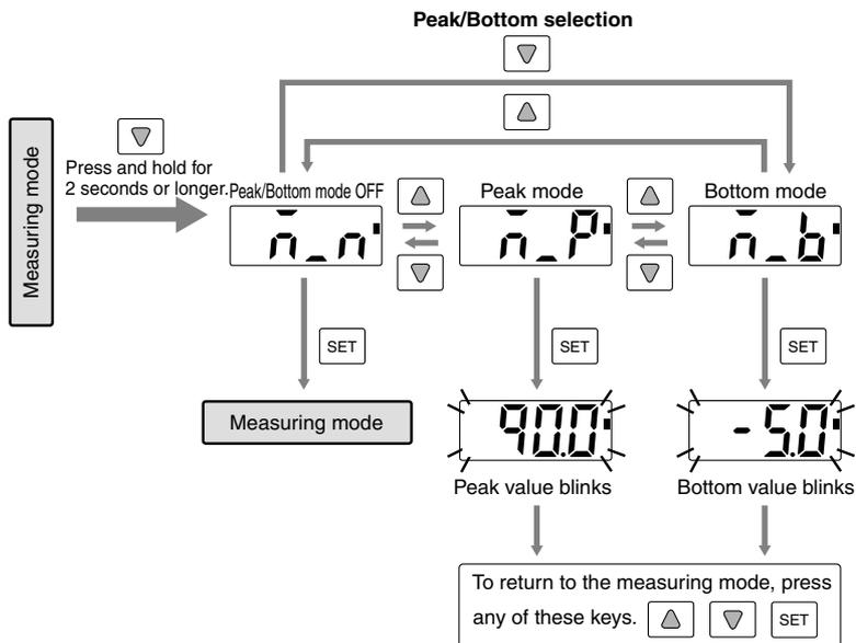
\* If any buttons other than above are pressed during the peak/bottom mode, the peak/bottom mode will be deactivated.
