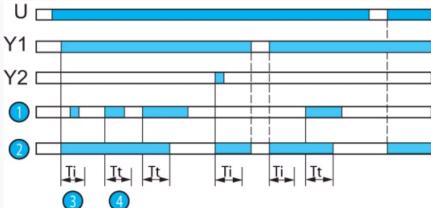
This mode is for controlling a pump based on one external signal (Y1). The relay output is closed when the signal is present at Y1 (contact closed). After a fault the relay remains open (even if the current returns to normal) and the module can be reclosed in two different ways : - By a reset : cutting of power supply,
