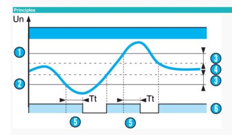
MUSF relays operate in window mode: they check that the controlled voltage stays between a minimum and maximum threshold. The under and overvoltage threshold values are set by two graduated potentiometers by reading the Un scale to be monitored directly. The hysteresis is fixed, value: 3 % of the preset thresholds.
