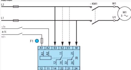
NB: When controlling DC voltage from the same source supplying terminals A1 and A2, terminal M must be connected directly to the "minus" pole of this power supply.
