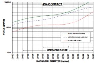
acteristics above were derived using 30 microinch gold plated contact and polished steel gauge pins having a bullet-shaped tip.
