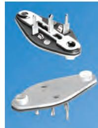
Easily assembles onto printed circuit board. Eliminates wiring. Stops on PC terminals provide sufficient spacing between socket and PC board to permit proper assembly of transistor to socket. Can be screwed down tightly to heat sink.
