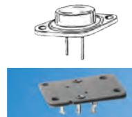
Socket and transistor are assembled to chassis at same time, using the minimum amount of hardware. Top molded boss ensure the transistor leads will be isolated from the chassis. Various boss heights available to accommodate different chassis thicknesses.
