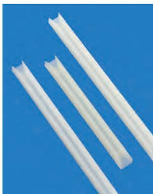
Guides may be used horizontally or vertically and snap into .125 (3.2) diameter holes. Narrow width allows maximum density and optimum airflow. Simple press-fit, secure installation.
