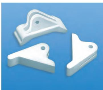
Designed for .062 (1.57) thick PC cards. Level action ejectors aids card insertion and extraction. Supplied complete with stainless steel spring pin.
