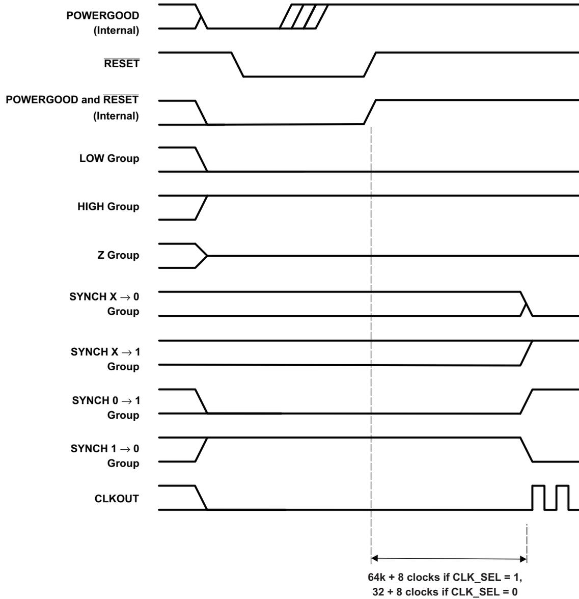
Figure 5-10. Reset Timing Requirements
