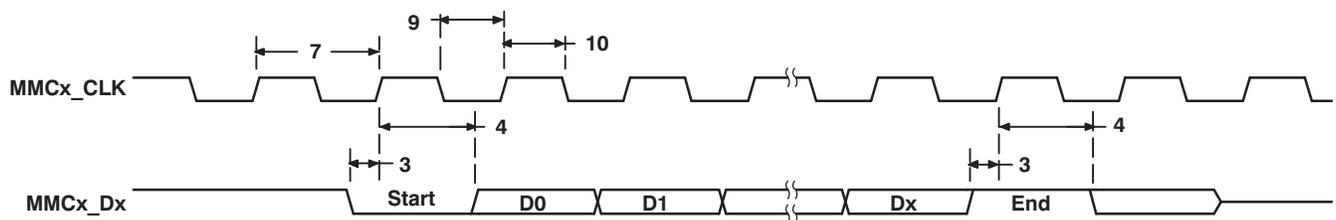
Figure 5-19. MMC/SD Card Response Timing
