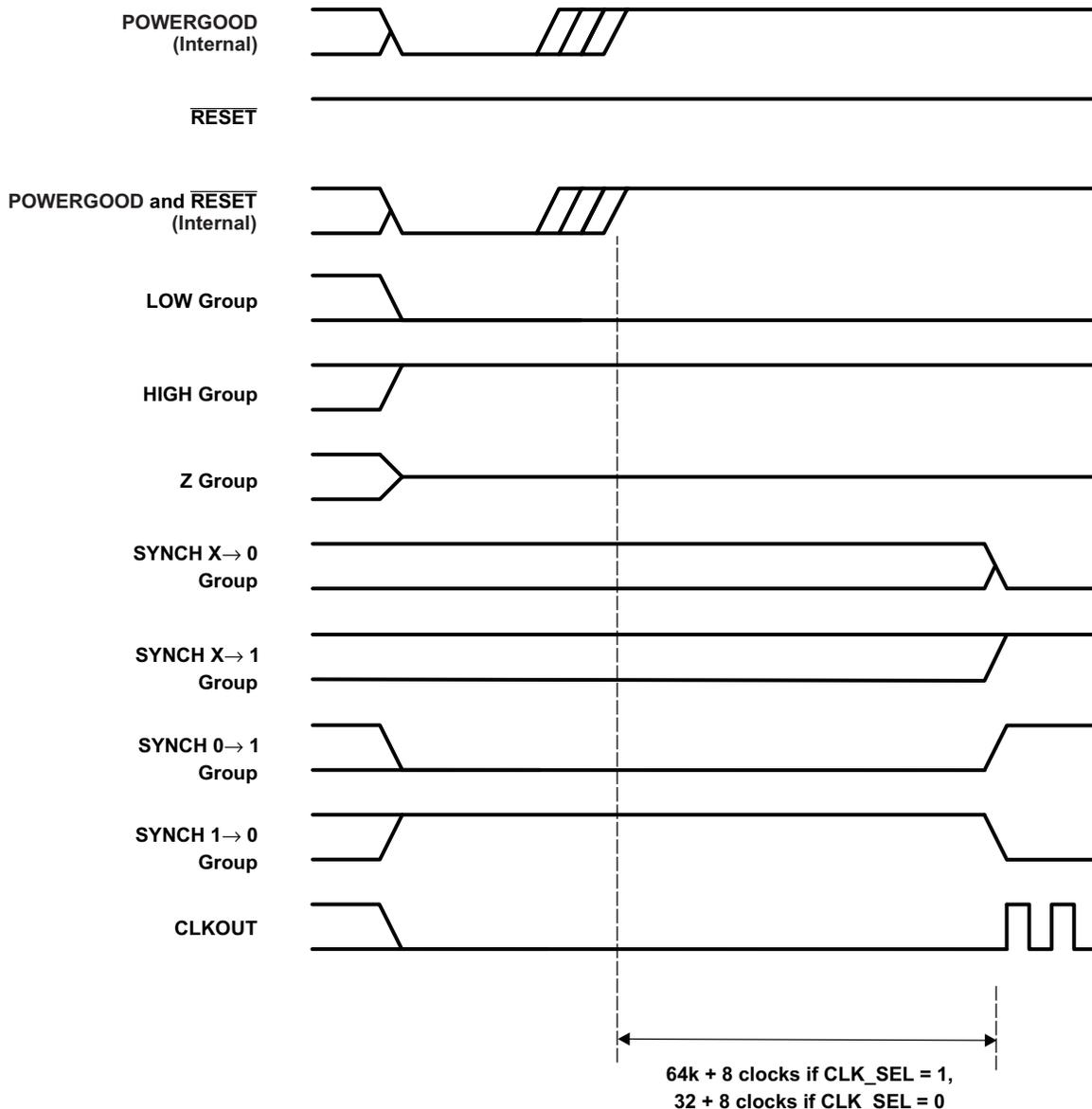
Figure 5-9. Power-On Reset Timing Requirements
