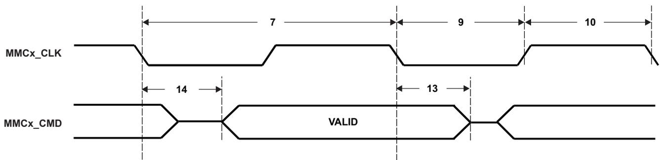
Figure 5-18. MMC/SD Host Command Write Timing
