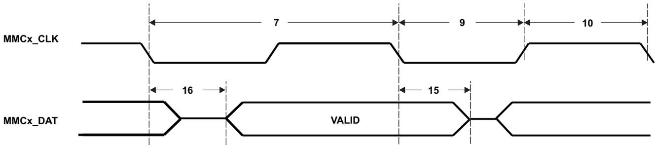
Figure 5-21. MMC/SD Data Write Timing
