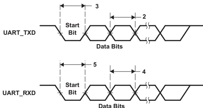
Figure 5-24. UART Transmit/Receive Timing
