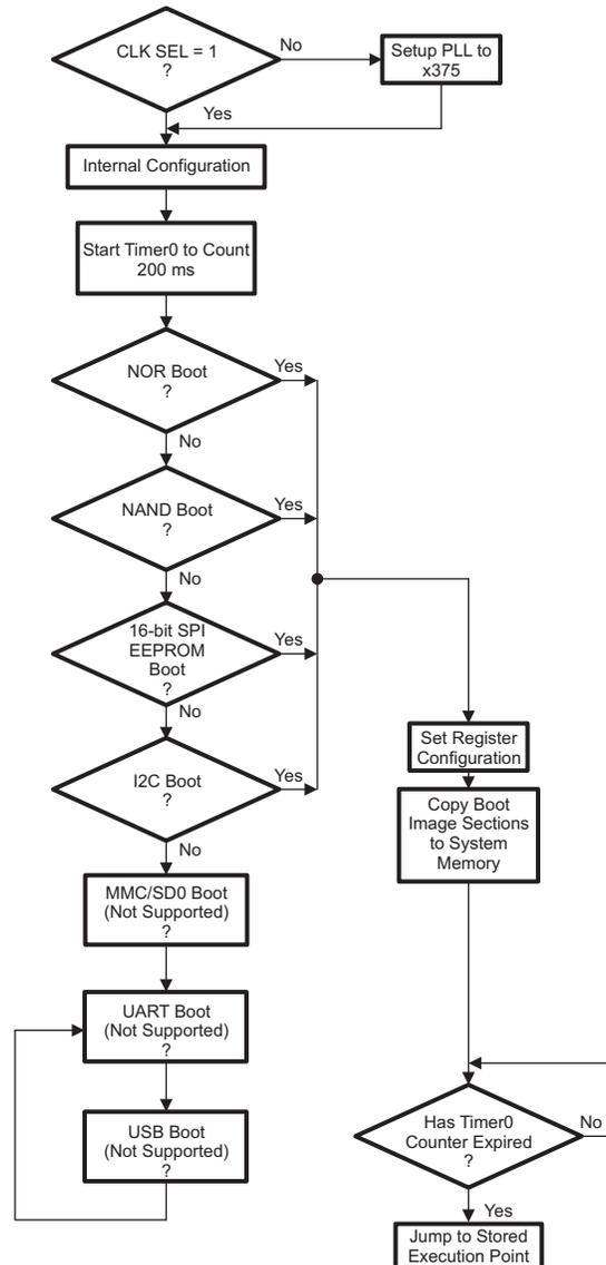
Figure 3-1. Bootloader Software Architecture
