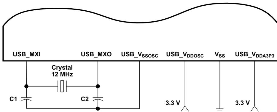
Figure 5-6. 12-MHz USB Oscillator
