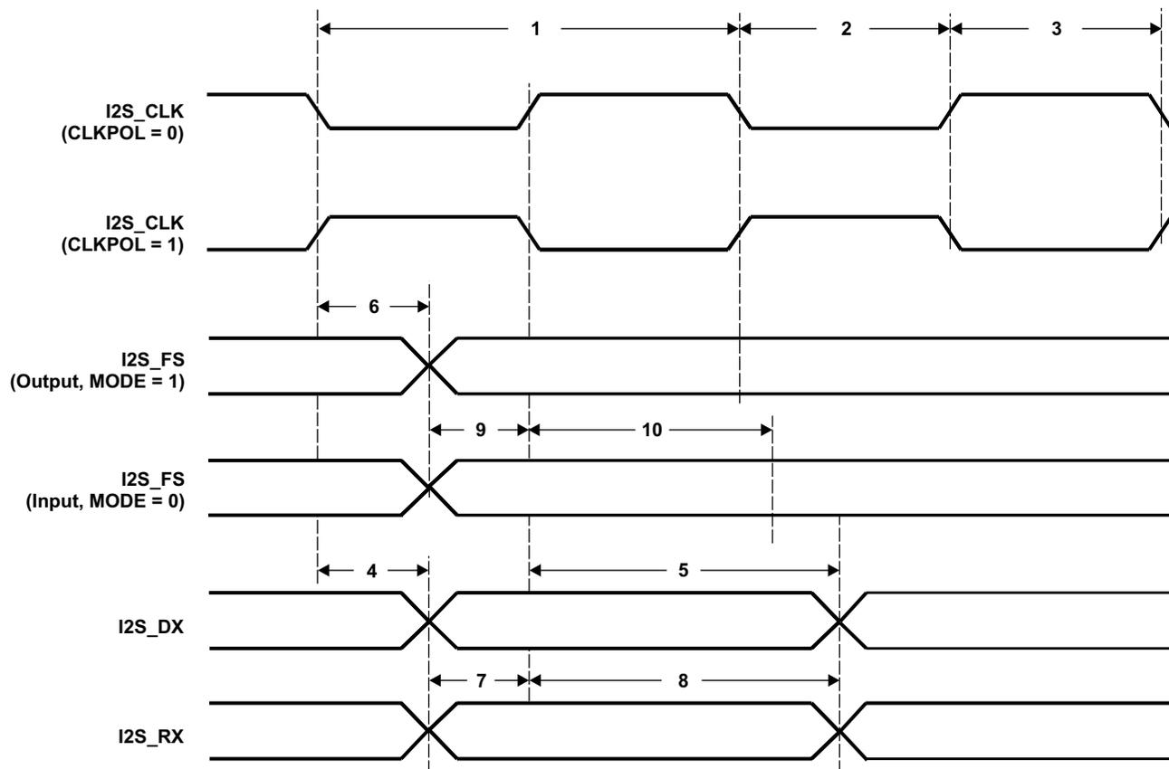
Figure 5-25. I2S Input and Output Timings
