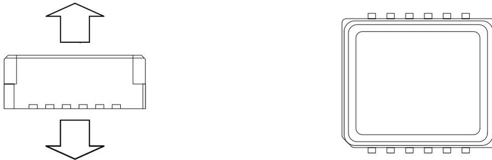
**Figure 3.** Accelerometer measuring directions
