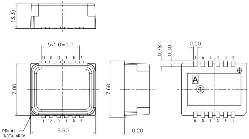
**Figure 2.** Housing dimensions
