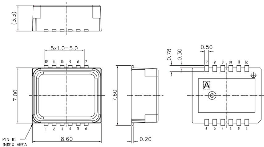
**Figure 3.** Housing dimensions
