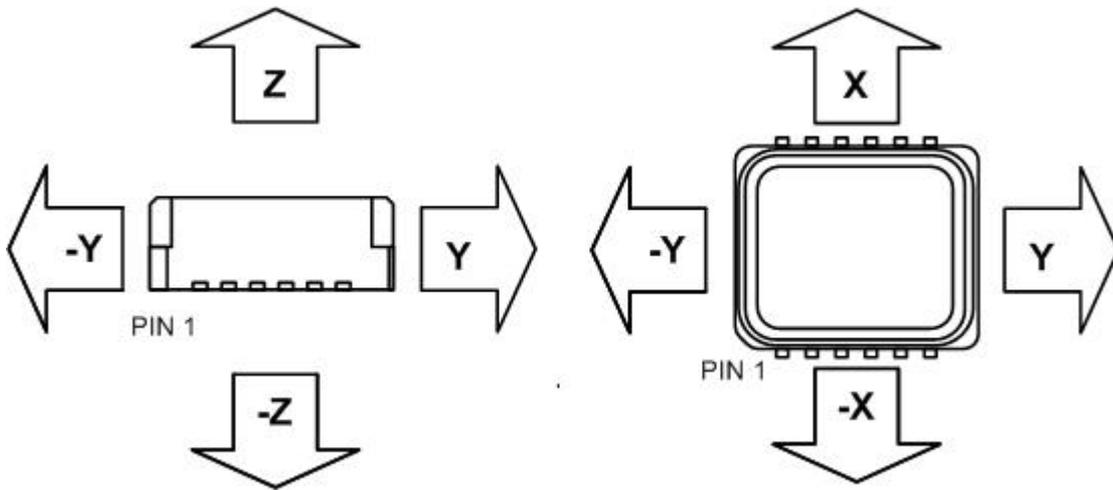
**Figure 2.** Accelerometer measuring directions
