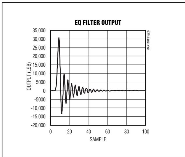
Figure 6. EQ Filter Response to a Step Input
