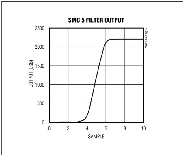
Figure 5. Sinc 5 Filter Response to a Step Input
