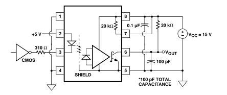
Figure 15. Recommended LED drive circuit.
