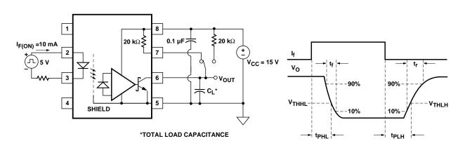
Figure 6. Propagation delay test circuit.
