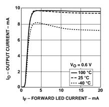
Figure 1. Typical transfer characteristics.
