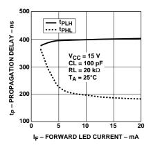
Figure 13. Propagation delay vs. input current.
