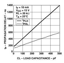
Figure 11. Propagation delay vs. load
