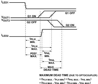
= (t<sub>PLH MAX.</sub> - t<sub>PLH MIN.</sub>) + (t<sub>PHL MAX.</sub> - t<sub>PHL MIN.</sub>) = (t<sub>PLH MAX.</sub> - t<sub>PHL MIN.</sub>) - (t<sub>PLH MIN.</sub> - t<sub>PHL MAX.</sub>) = PDD\* MAX. - PDD\* MIN.
