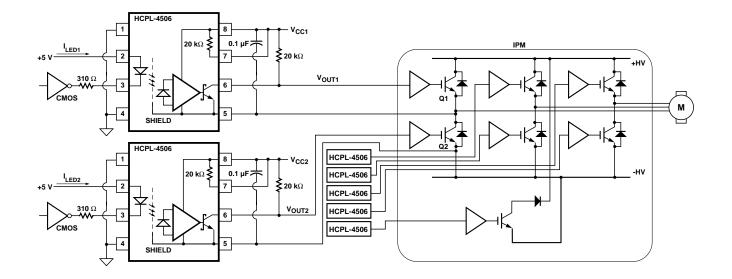
Figure 24. Typical application circuit.
