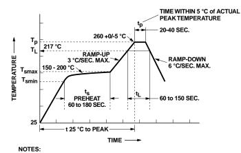
THE TIME FROM 25 °C to PEAK TEMPERATURE = 8 MINUTES MAX. T<sub>smax</sub> = 200 °C, T<sub>smin</sub> = 150 °C
