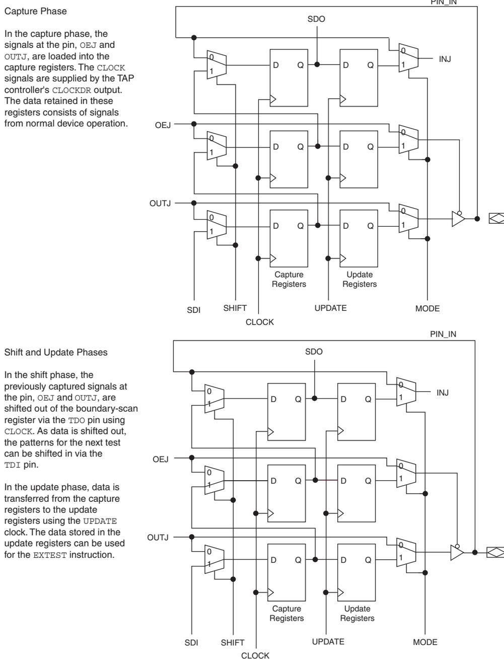
During the capture phase, multiplexers preceding the capture registers select the active device data signals. This data is then clocked into the capture registers. The multiplexers at the outputs of the update registers also select active device data to prevent functional interruptions to the device. During the shift phase, the boundary-scan shift register is formed by clocking data through the capture registers
