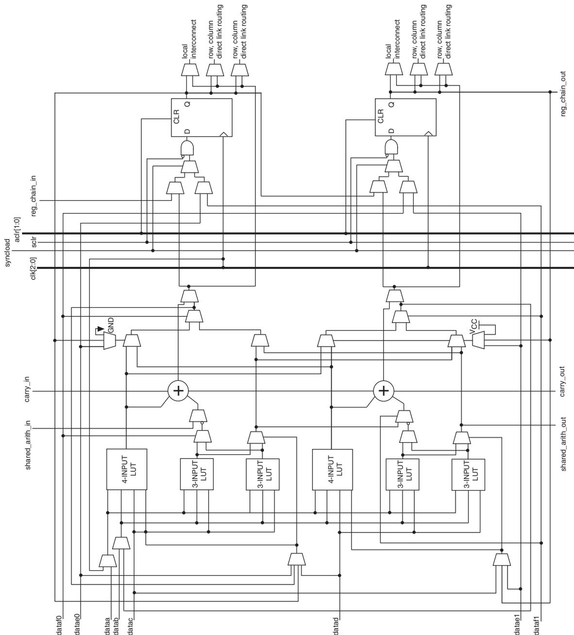
One ALM contains two programmable registers. Each register has data, clock, clock enable, synchronous and asynchronous clear, and synchronous load/clear inputs. Global signals, general-purpose I/O pins, or any internal logic can drive the register's clock and clear control signals. Either general-purpose I/O pins or internal logic can drive the clock enable. For combinational functions, the register is bypassed and the output of the LUT drives directly to the outputs of an ALM.
