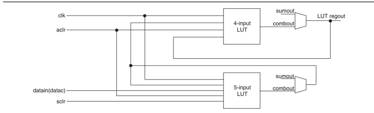
**Figure 2-16.** ALM in LUT-Register Mode with 3-Register Capability
