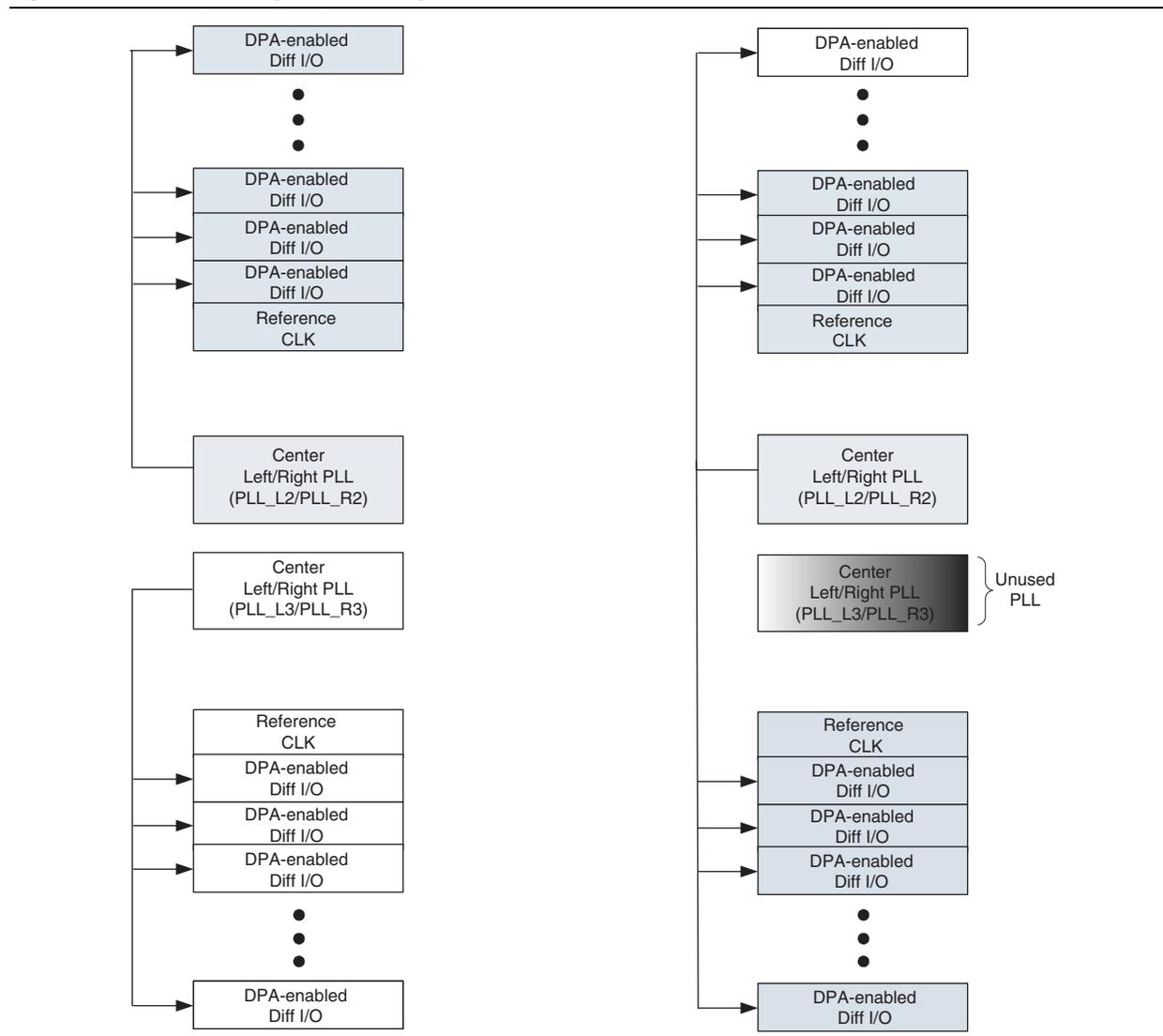
**Figure 9-21.** Invalid Placement of DPA-Enabled Differential I/Os Driven by Both Center Left/Right PLLs
