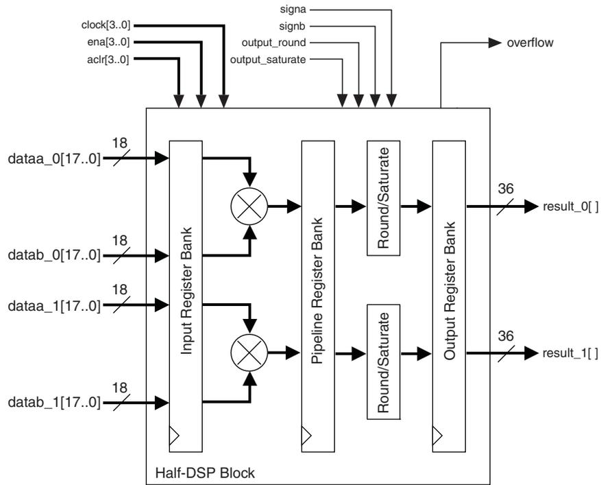
**Figure 5-9.** 12-Bit Independent Multiplier Mode Shown for Half-DSP Block
