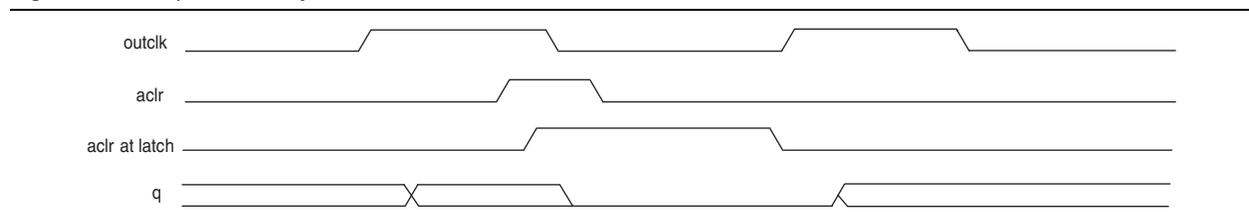
You can selectively enable asynchronous clears per logical memory via the Quartus II RAM MegaWizard® Plug-In Manager.
