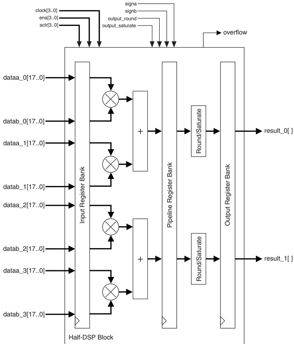
Figure 5-15. Loopback Mode for Half-DSP Block
