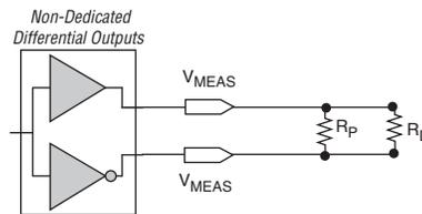
**Figure 1-7.** Output Delay Timing Reporting Setup modeled by Quartus II Software for Differential Outputs with Three External Resistor
