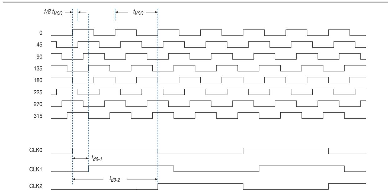
You can use the coarse- and fine-phase shifts to implement clock delays in Stratix III devices.
