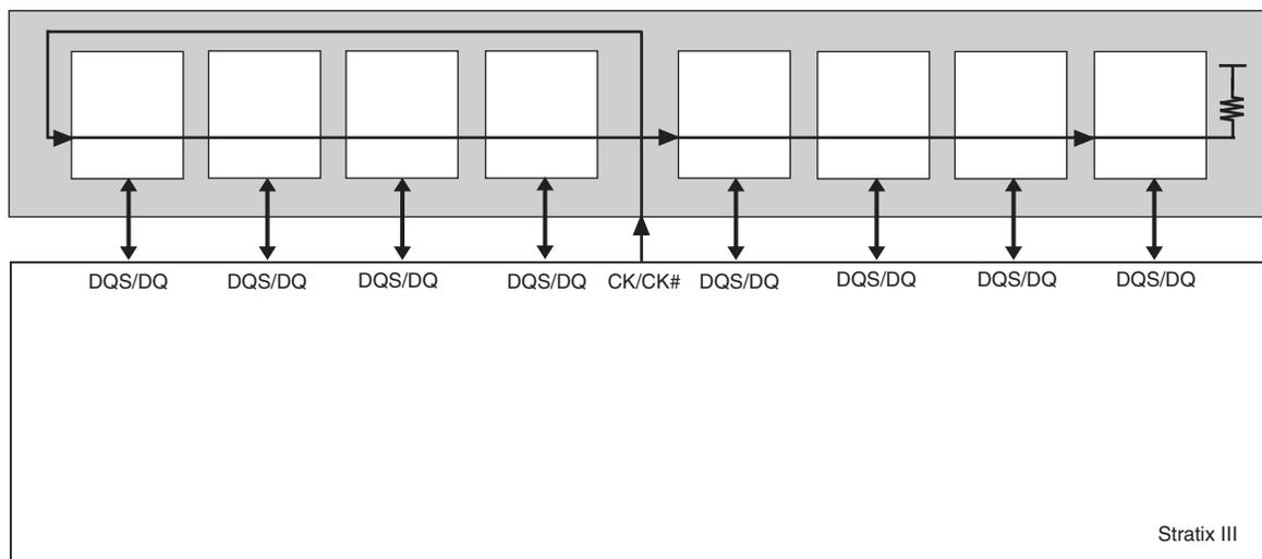
Because the data and read strobe signals are still point-to-point, special consideration needs to be taken to ensure that the timing relationship between CK/CK# and DQS signals ( $t_{DQSS}$ ) during a write is met at every device on the modules. Furthermore, read data coming back into the FPGA from the memory is also staggered in a similar way.
