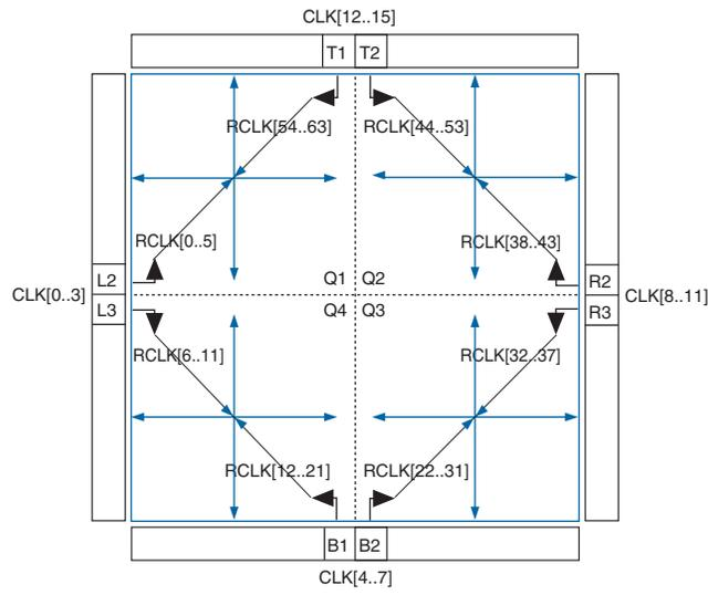
**Figure 6-4.** Regional Clock Networks (EP3SL200, EP3SE260, and EP3SL340 Devices) *(Note 1)*
