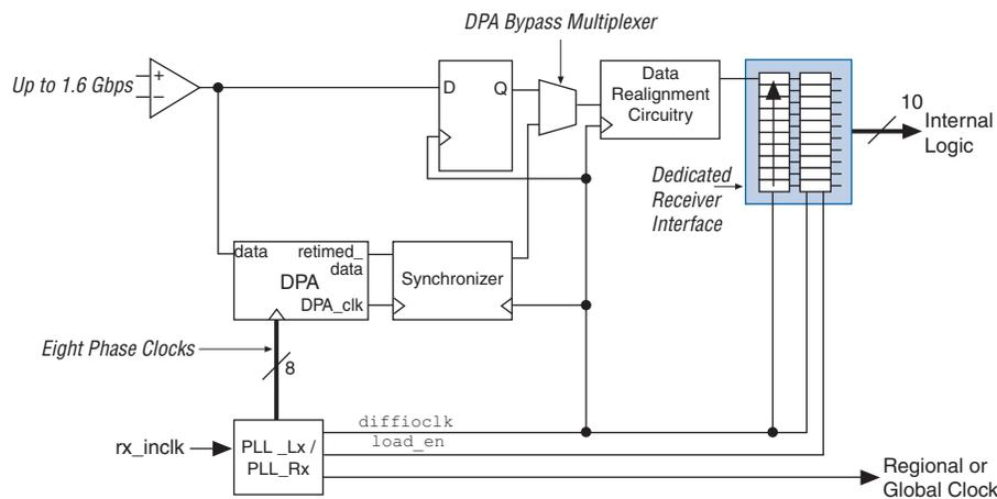
Figure 9-6 shows the deserializer bypass data path.
