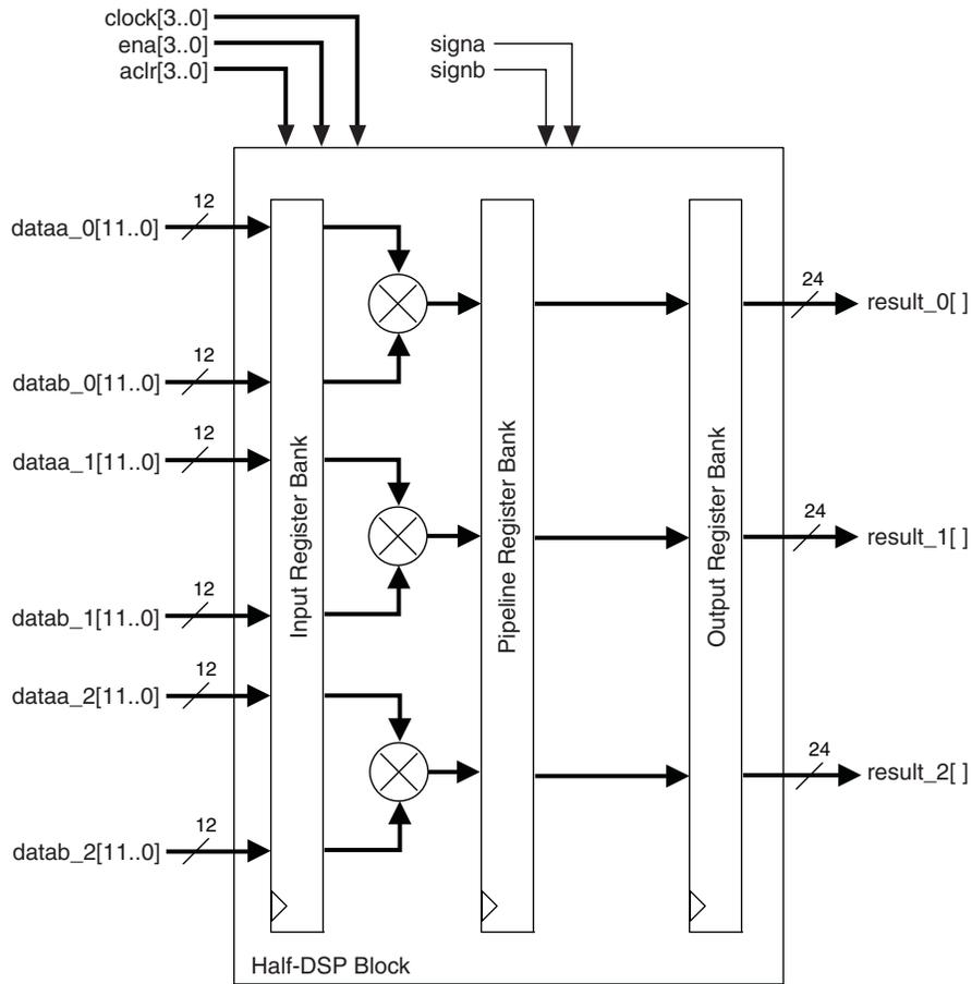
Figure 5-10. 9-Bit Independent Multiplier Mode Shown for Half-Block
