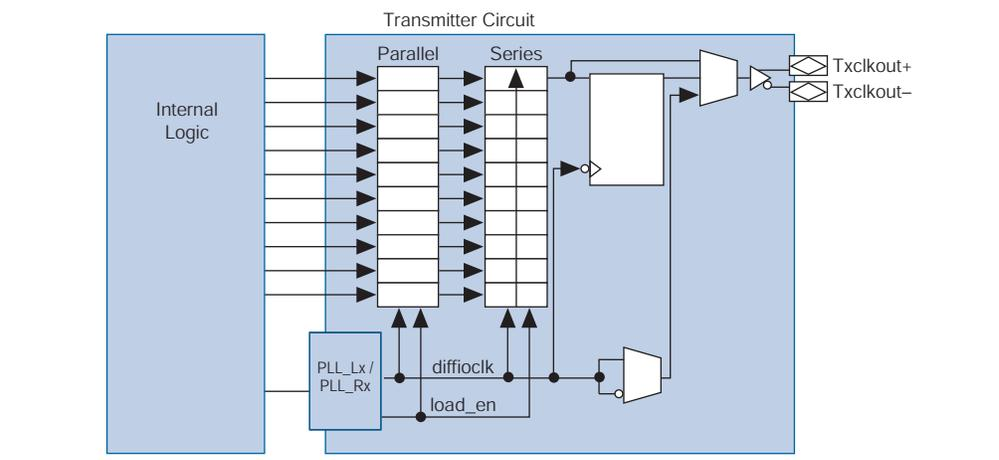
The Stratix III serializer can be bypassed to support DDR (×2) and SDR (×1) operations to achieve a serialization factor of 2 and 1, respectively. The I/O element (IOE) contains two data output registers that can each operate in either DDR or SDR mode. The clock source for the registers in the IOE can come from any routing resource, from the left/right PLL (PLL\_Lx/PLL\_Rx) or from the top/bottom (PLL\_Tx/PLL\_Bx) PLL. Figure 9-4 shows the serializer bypass path.
