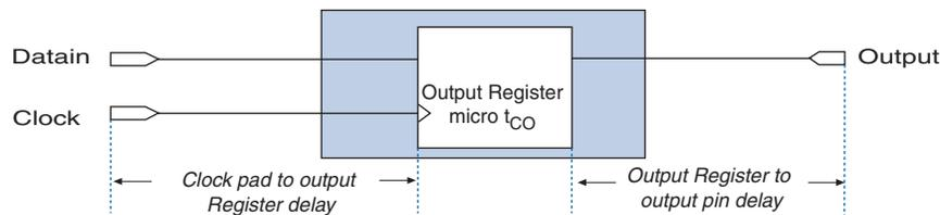
Simulation using IBIS models is required to determine the delays on the PCB traces in addition to the output pin delay timing reported by the Quartus II software and the timing model in the device handbook.
