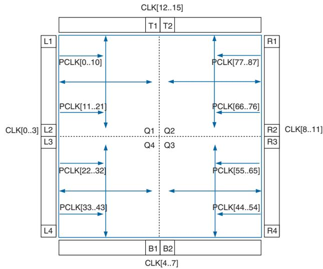
Figure 6-8. Periphery Clock Networks (EP3SE260 Devices)
