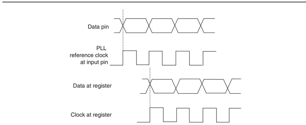
**Figure 6-27.** Phase Relationship Between Clock and Data LVDS Modes
