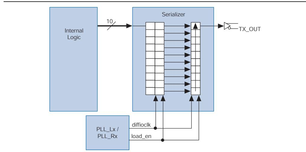
Any Stratix III transmitter data channel can be configured to generate a source synchronous transmitter clock output. This flexibility allows placing the output clock near the data outputs to simplify board layout and reduce clock-to-data skew. Different applications often require specific clock-to-data alignments or specific data rate to clock rate factors. The transmitter can output a clock signal at the same rate as the data with a maximum frequency of 717 MHz. The output clock can also be
