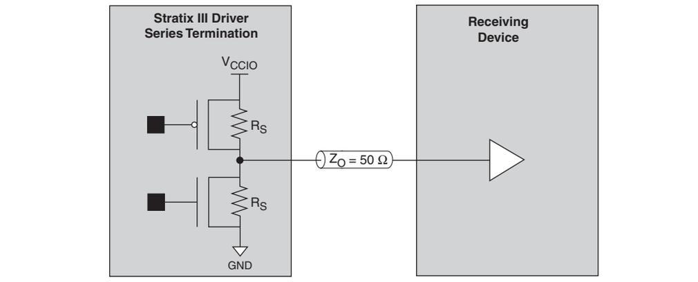
To use on-chip termination for the SSTL Class I standard, you should select the **50- $\Omega$  on-chip series termination** setting, eliminating the external 25- $\Omega$   $R_S$  (to match the 50- $\Omega$  transmission line). For the SSTL Class II standard, you should select the 25- $\Omega$  on-chip series termination setting (to match the 50- $\Omega$  transmission line and the near-end external 50- $\Omega$  pull-up to  $V_{TT}$ ).
