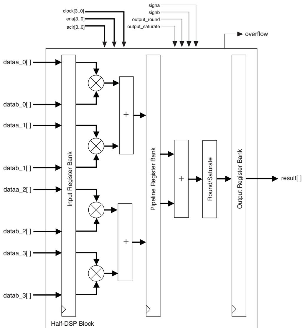
The four-multiplier adder mode supports the round and saturation logic unit. You can use the pipeline registers and output registers within the DSP block to pipeline the multiplier-adder result, increasing the performance of the DSP block.
