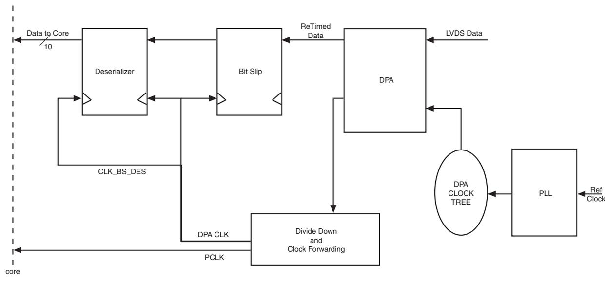
Note that the synchronizer FIFO is bypassed in soft-CDR mode. The reference clock frequency must be suitable for the PLL to generate a clock that matches the data rate of the interface. The DPA circuitry can track PPM differences between the reference clock and the data stream.
