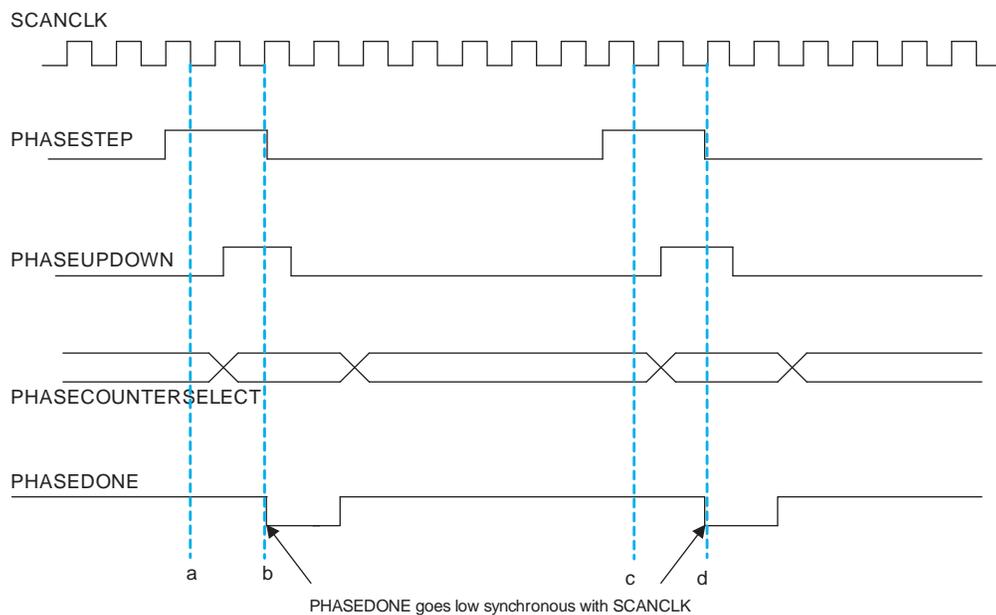
Dynamic phase-shifting can be repeated indefinitely. All signals are synchronous to scanclk and must meet  $t_{su}/t_h$  requirements with respect to scanclk edges.
