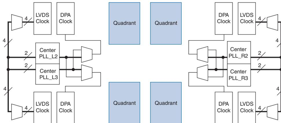
**Figure 9-14.** LVDS/DPA Clocks in Stratix III Devices with Center and Corner PLLs
