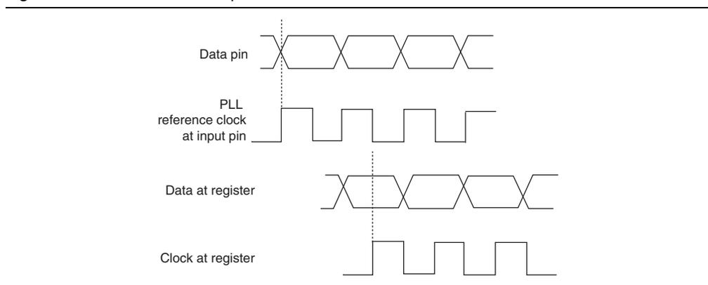
The source-synchronous mode compensates for the delay of the clock network used plus any difference in the delay between these two paths:
