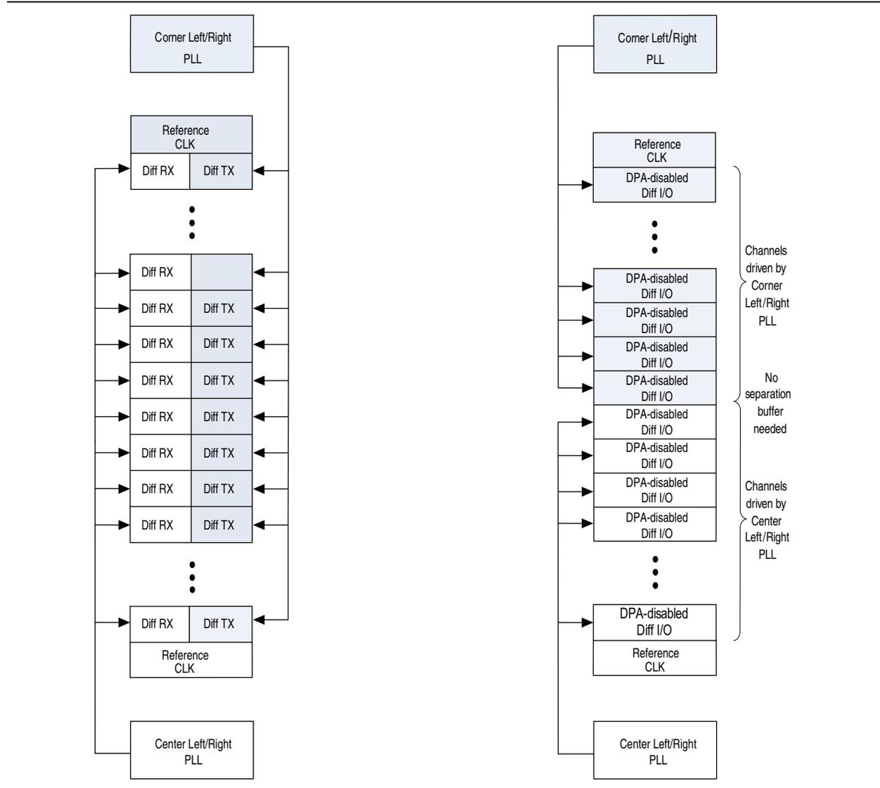
**Figure 9-23.** Invalid Placement of DPA-Disabled Differential I/Os Due to Interleaving of Channels Driven by the Corner and Center Left/Right PLLs
