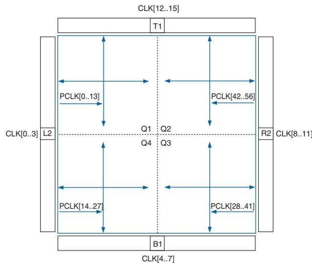
**Figure 6-6.** Periphery Clock Networks (EP3SL110, EP3SL150, EP3SE80, and EP3SE110 Devices)
