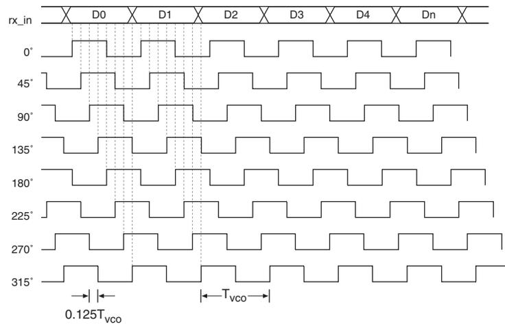
The DPA block continuously monitors the phase of the incoming serial data and selects a new clock phase if needed. You can prevent the DPA from selecting a new clock phase by asserting the optional `RX_DPLL_HOLD` port, which is available for each channel.
