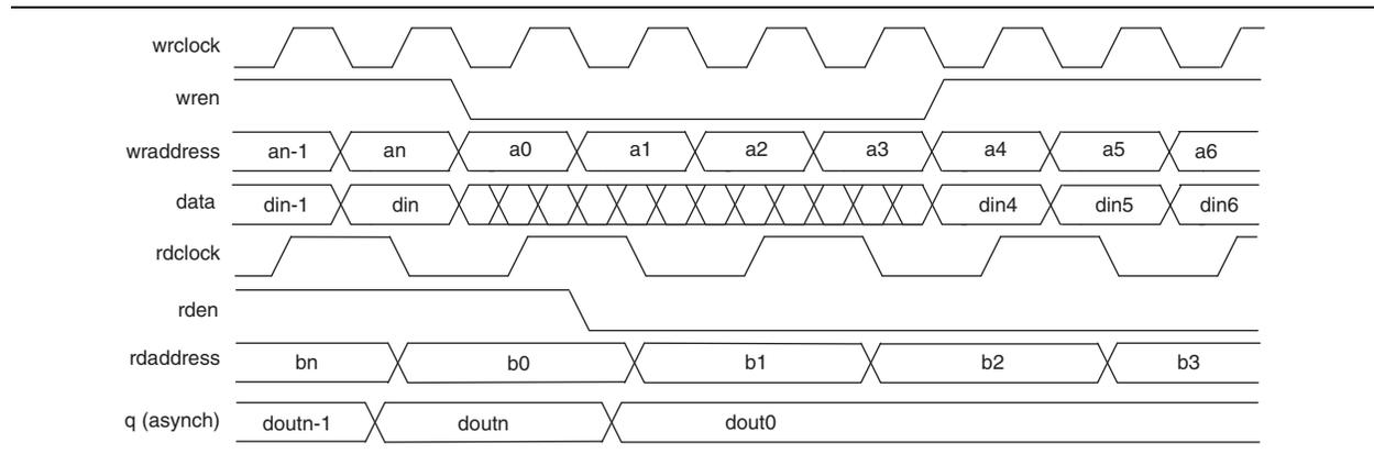
Figure 4-11 shows timing waveforms for read and write operations in mixed-port mode with unregistered outputs.
