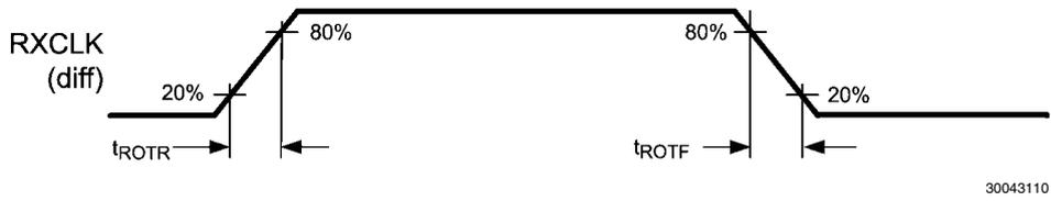
FIGURE 2. LVDS Output Transition Time
