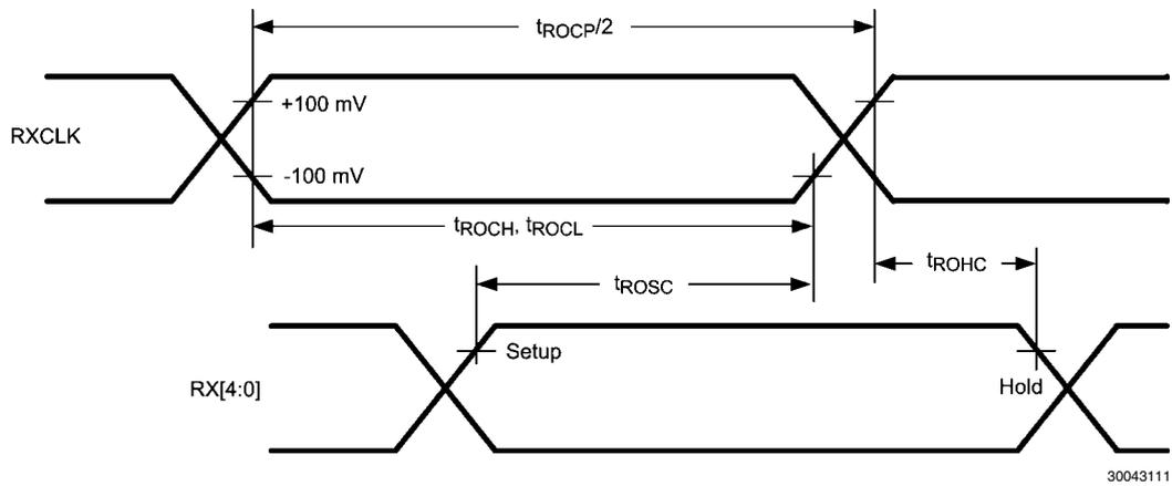
FIGURE 3. Deserializer (LVDS Interface) Setup/Hold and High/Low Times
