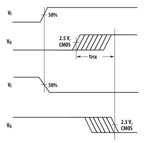
Figure 9. Propagation delay skew waveform
