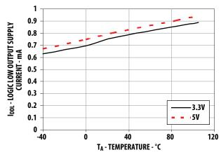
Figure 4. Typical logic low output supply current versus temperature.
