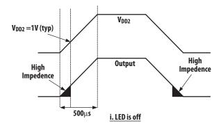
Figure 13. V<sub>DD</sub> Ramp when LED is off.
