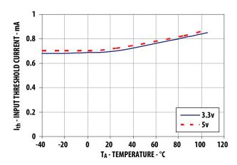
Figure 2. Typical input threshold current versus temperature.
