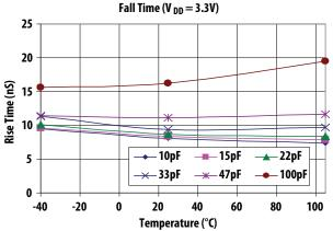
Figure 15. Rise and Fall time of ACPL-x6xL across wide load capacitance
