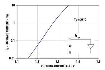
Figure 1. Typical input diode forward current characteristic.
