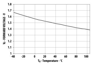
Figure 7. Typical V<sub>F</sub> versus temperature.
