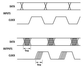
Figure 10. Parallel data transmission example
