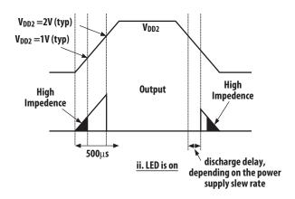
Figure 14. V<sub>DD</sub> Ramp when LED is on.
