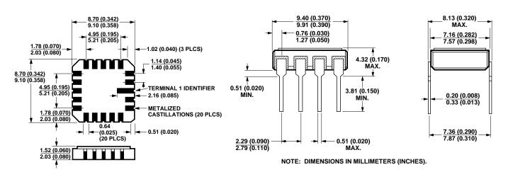
NOTE: DIMENSIONS IN MILLIMETERS (INCHES). SOLDER THICKNESS 0.127 (0.005) MAX.
