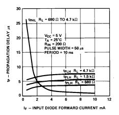
Figure 7. Propagation Delay vs. Input Diode Forward Current.
