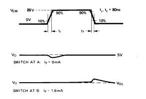
Figure 9. Test Circuit for Transient Immunity and Typical Waveforms.
