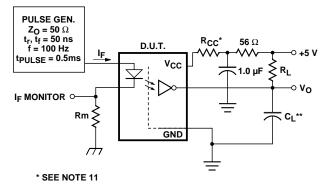
\*\* CLINCLUDES PROBE AND STRAY WIRING CAPACITANCE.
