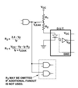
Figure 10. Recommended Drive Circuitry Using TTL Open-Collector Logic.
