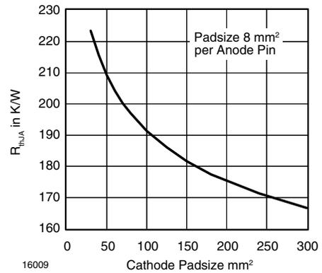
Figure 14. Thermal Resistance Junction Ambient vs. Cathode Padsize
