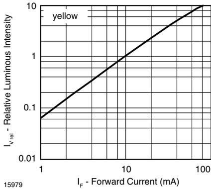
Figure 9. Relative Luminous Flux vs. Forward Current
