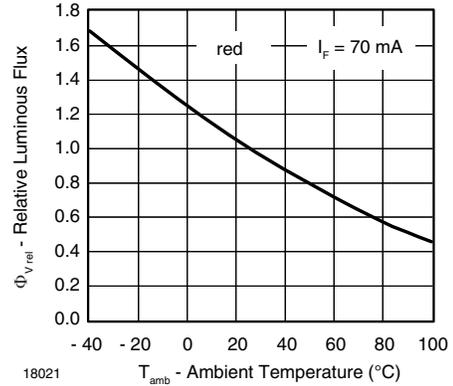
Figure 12. Rel. Luminous Flux vs. Ambient Temperature
