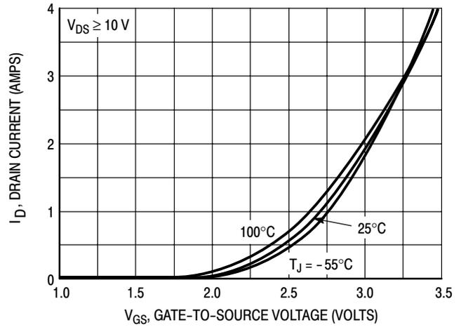
Figure 2. Transfer Characteristics
