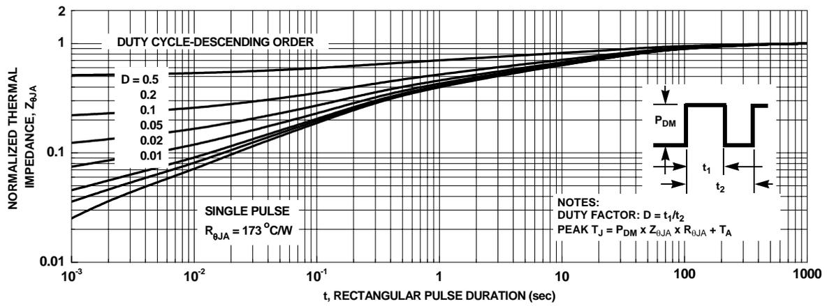
**Figure 12. Junction to Ambient Transient Thermal Response Curve**
