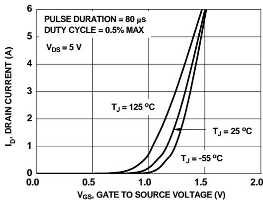
**Figure 5. Transfer Characteristics**
