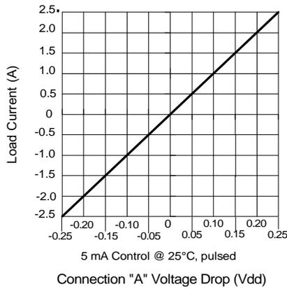
**Figure 3. Linearity Characteristics**
