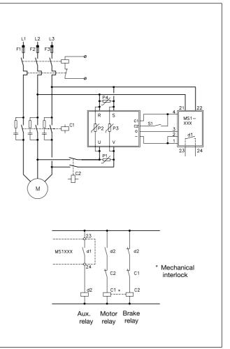
The MS1.. power supply connected to a motor controller (RRC) for reversing of an induction motor.
