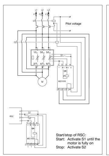
The MS1.. power supply connected to a motor controller (RTC) for dynamic braking of an induction motor.
