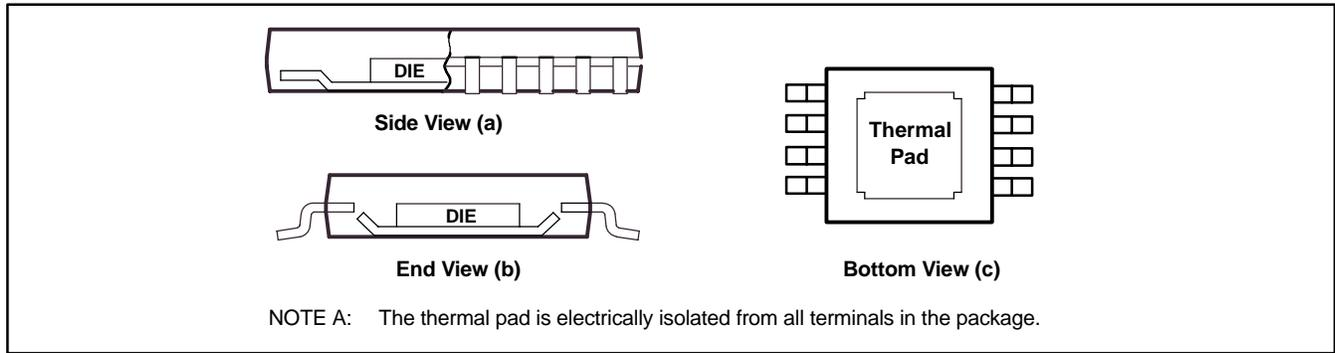
**Figure 51. Views of Thermally Enhanced DGN Package**
