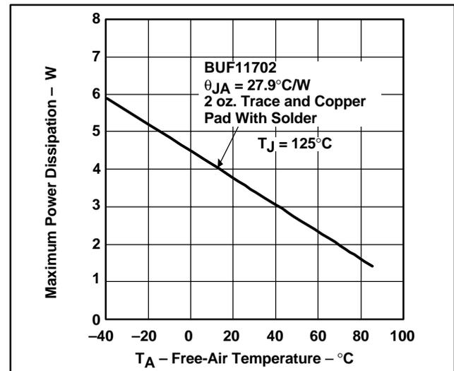
**Figure 52. Maximum Power Dissipation vs Free-Air Temperature**
