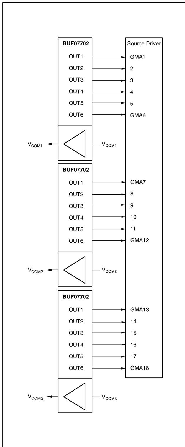
**Figure 49. 18-Channel Application with Five Integrated  $V_{COM}$  Channels**
