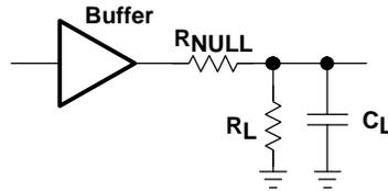
Figure 1. Bandwidth and Phase Shift Test Circuit
