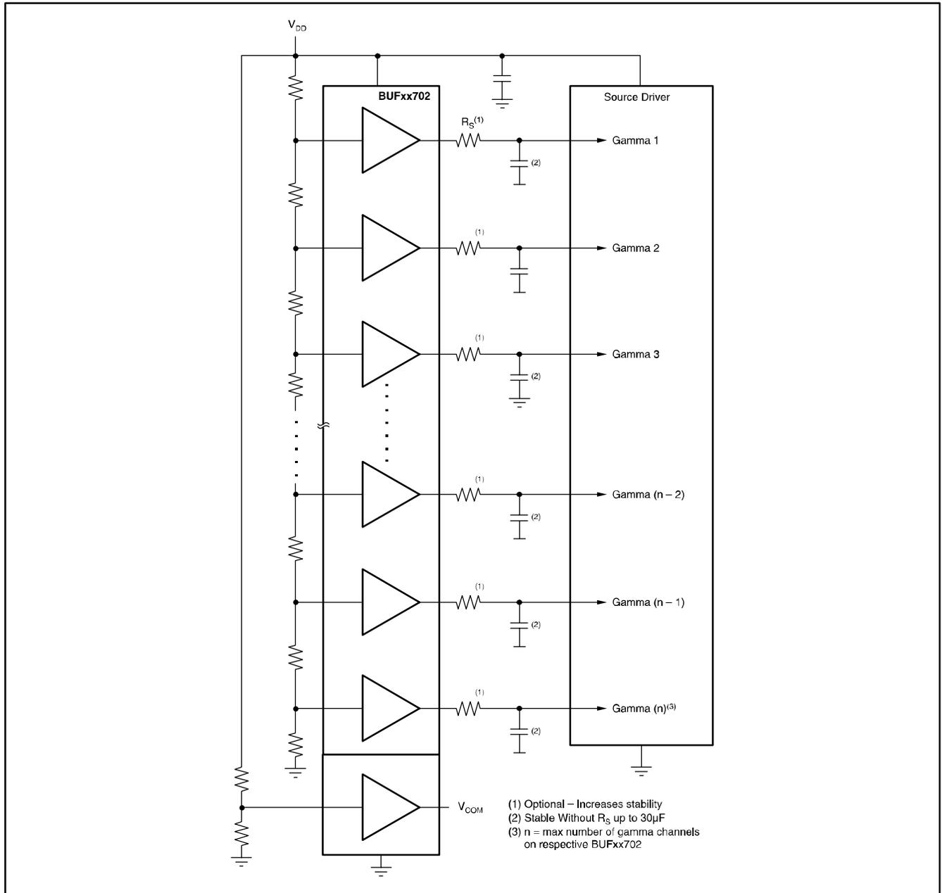
Figure 44. LCD Source Driver Typical Block Diagram
