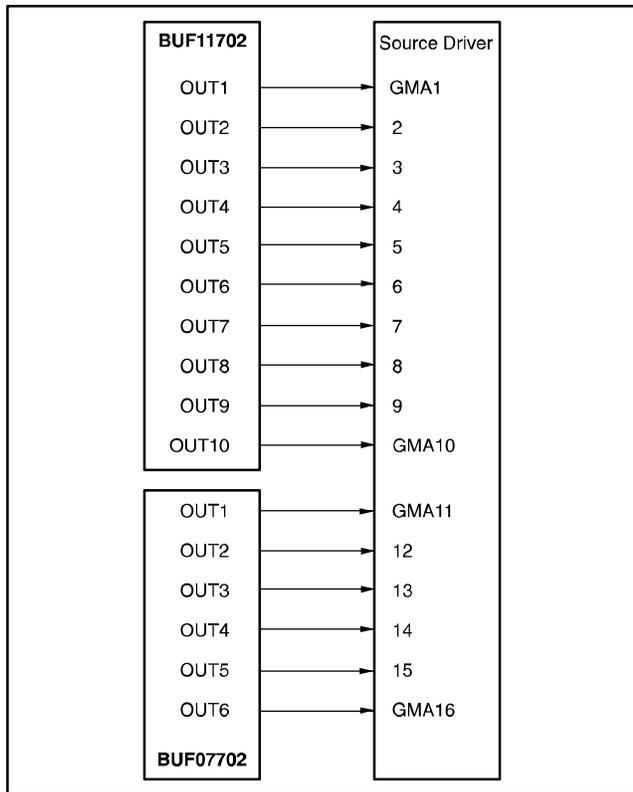
**Figure 48. Creating > 10 Gamma Voltage Channels**
