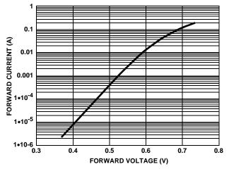
FIGURE 14. BOOTSTRAP DIODE I-V CHARACTERISTICS
