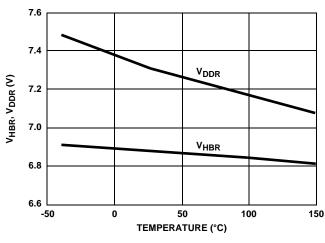
FIGURE 9. UNDERVOLTAGE LOCKOUT THRESHOLD vs TEMPERATURE
