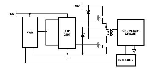
FIGURE 1. TWO-SWITCH FORWARD CONVERTER
