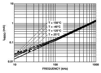
FIGURE 6. HB TO VSS OPERATING CURRENT vs FREQUENCY
