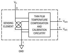
Figure 1. Temperature Compensated Pressure Sensor Schematic
