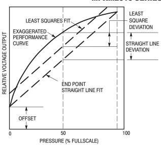
Figure 2. Linearity Specification Comparison
