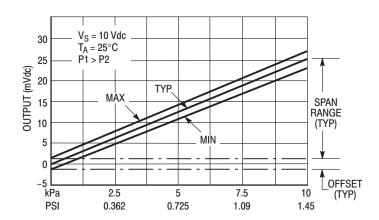
Figure 3. Output versus Pressure Differential
